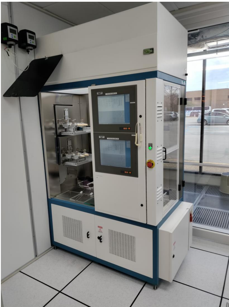
Figure 3: Tystar Oxidation Furnace for Thermal Oxidation of Silicon
