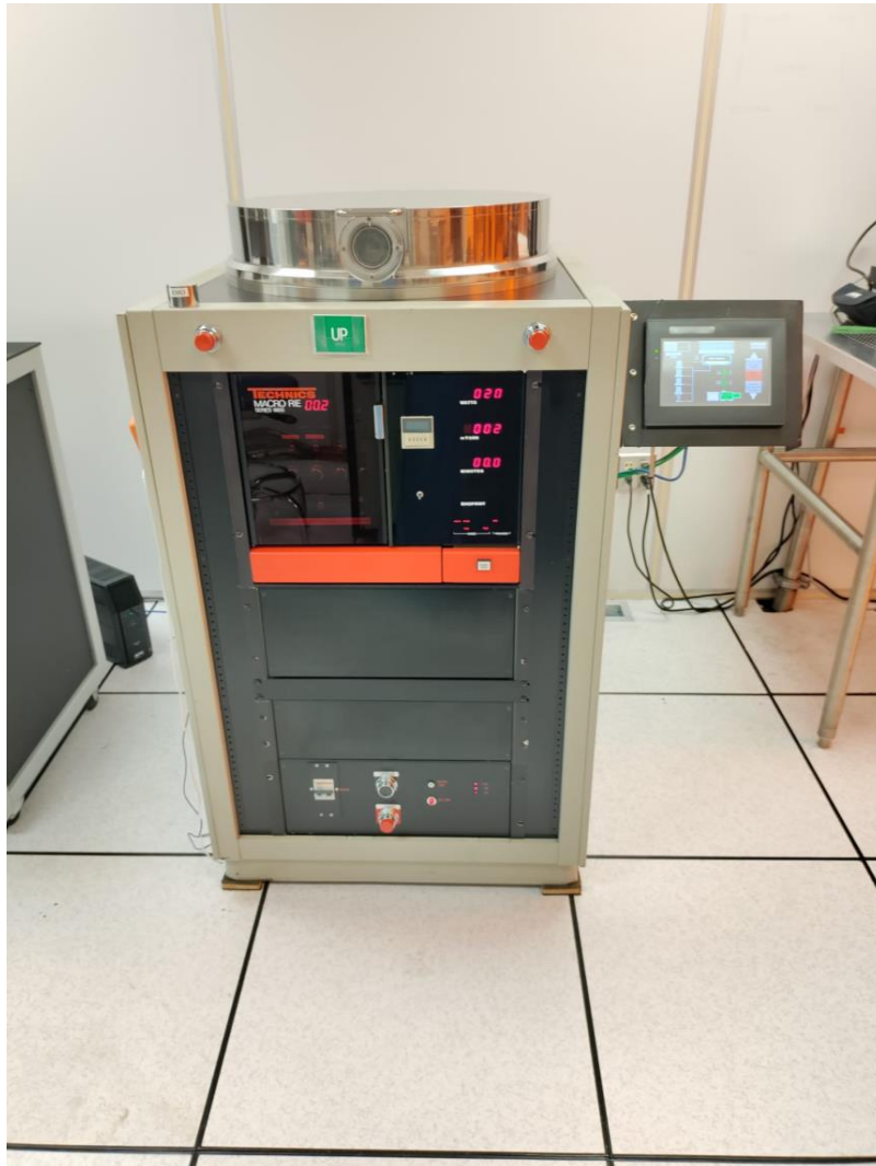
Figure 6: Technics Macro RIE – 8800 equipment for Reactive Ion Etching
