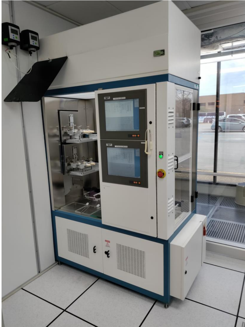
Figure 22: Tystar Oxidation Furnace for Thermal Oxidation of Silicon
