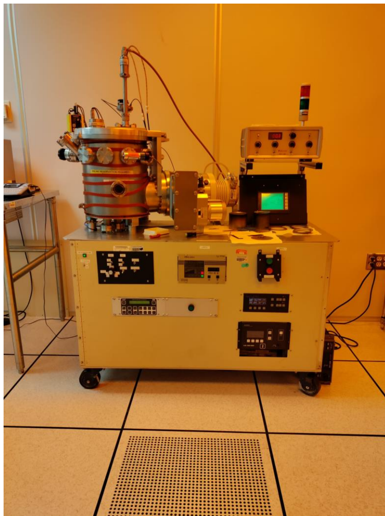
Figure 26: Homebuilt Sputter deposition equipment for DC and RF Sputter deposition
