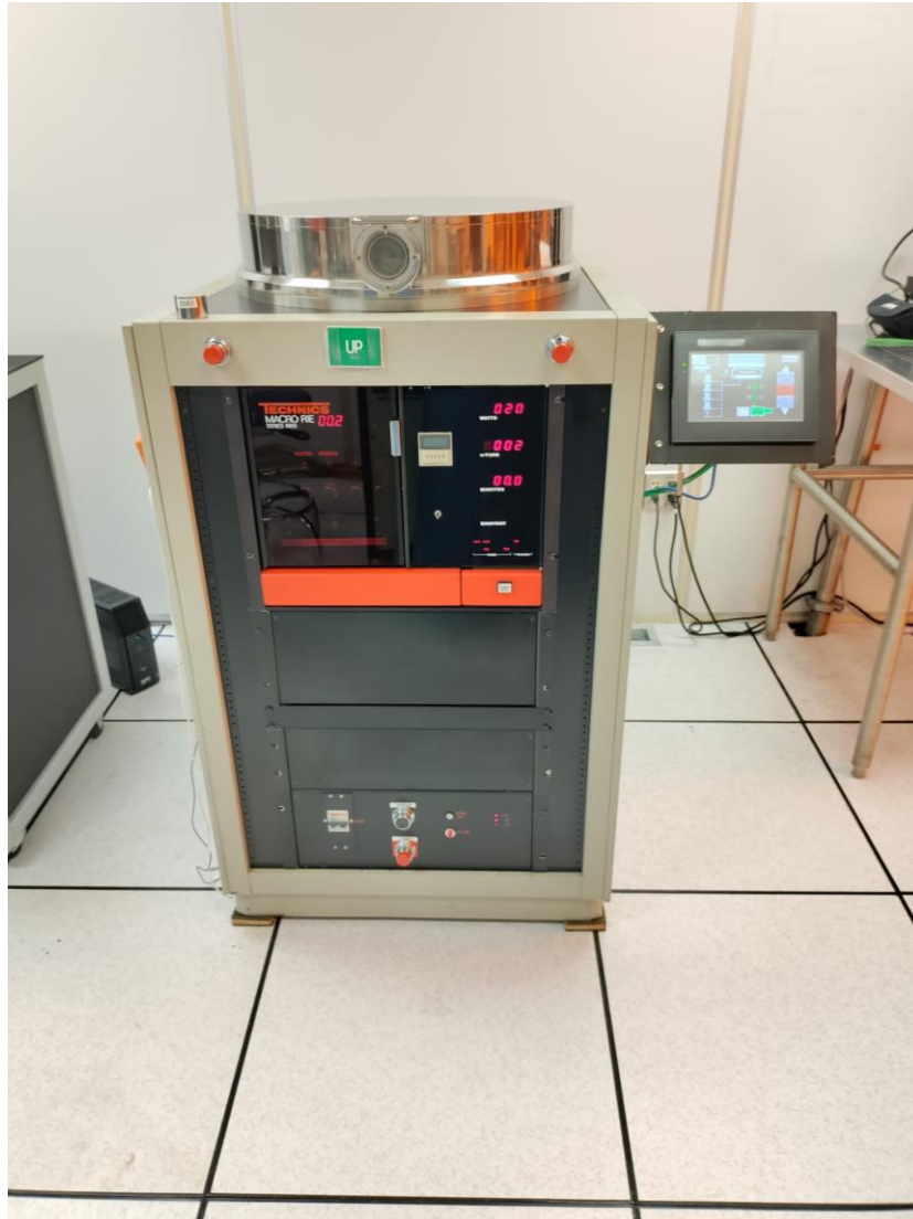
Figure 25: Technics Macro RIE – 8800 equipment for Reactive Ion Etching
