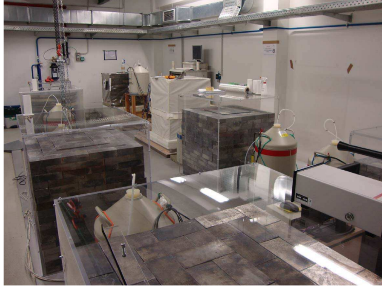
FIGURE 3.3: Left: Radioassay results from the original cathode we made whose manufacturers we are likely to go through again. Right: Laboratory at LSC with germanium detectors inside shielding[21] which performed the radiopurity screening shown left.
