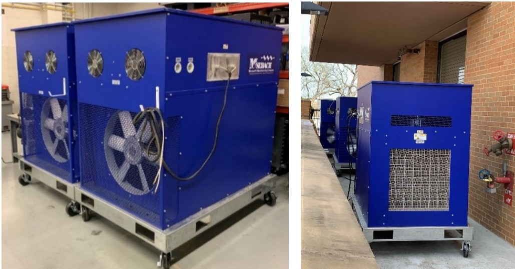
Figure 1.10: Photograph of the two 6 kVDC – 150-kW resistive loads (left) and all three load banks lined up in operational state (right).
