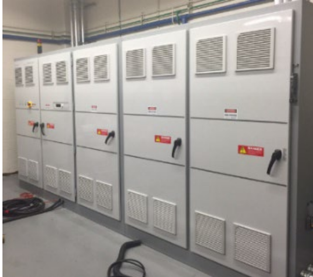
Figure 1.13: Photograph of UTA's 1200V/700A/500kW Chroma 17030 cycler.
