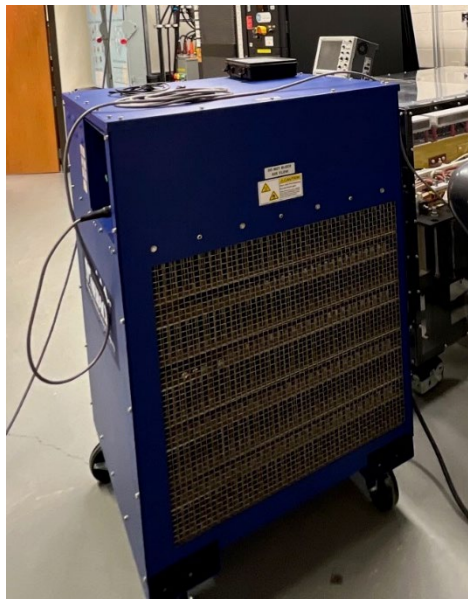
Figure 1.8: Photograph of the 480 VAC load.
