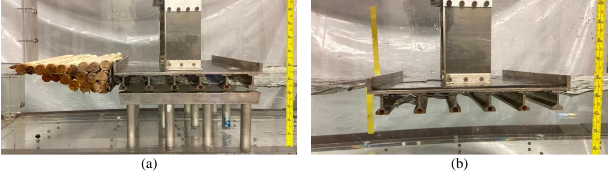
Fig. 4.15 Experimental setup for test series: (a) substructure-debris-superstructure (SDS) and (b) superstructure-only (SO)
