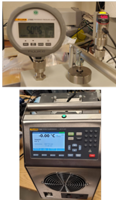
Figure 5-10: Pneumatic pressure calibration gauge (top) and temperature sensor calibration bath (bottom) used for pressure sensors and thermocouples
