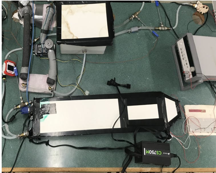
Figure 3-3: Experimental setup showing the server cooling loop, pump control circuitry, and instrumentation for data acquisition
