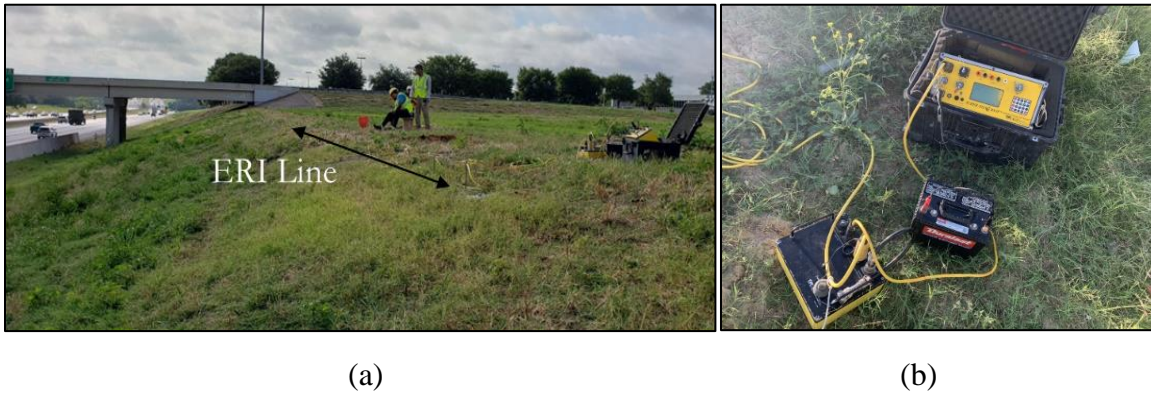
Figure 3-9 (a) Location of ERI line (b) 8 Channel SuperSting Equipment.
