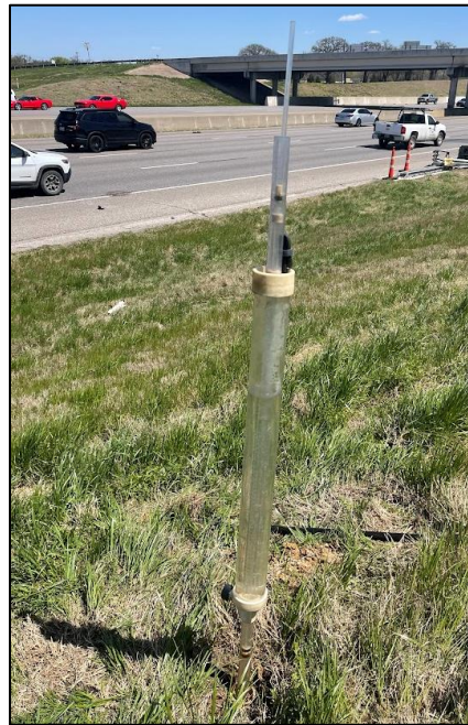
Figure 4-11 Instrumental Setup of Guelph Permeameter.
