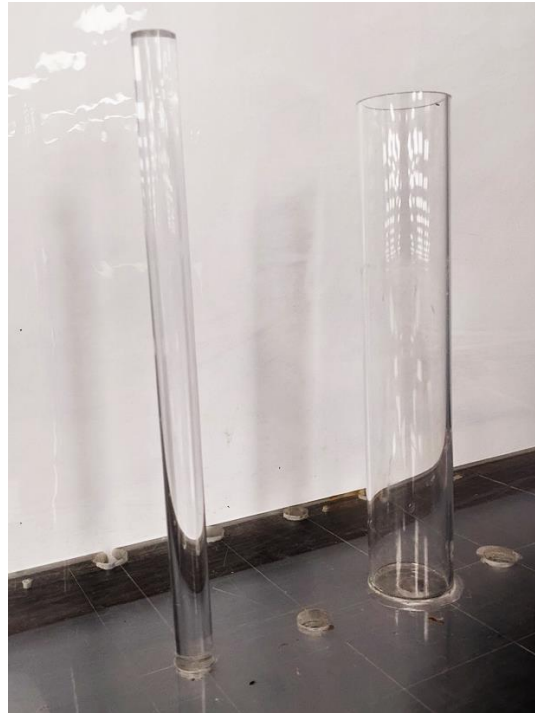
Figure 3.2. The 19 mm and 50 mm piers used in this study
