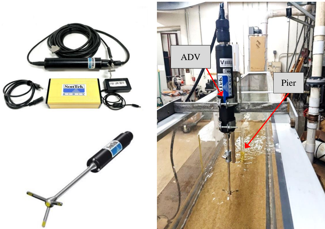
Figure 3.5. Acoustic doppler velocimeter (ADV) used to measure the velocity
