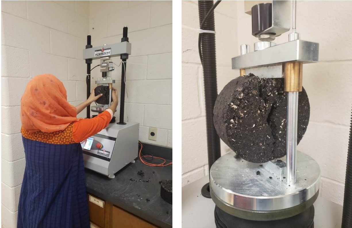
Figure 3.17. Test Set-Up for Indirect Tensile Strength Test
