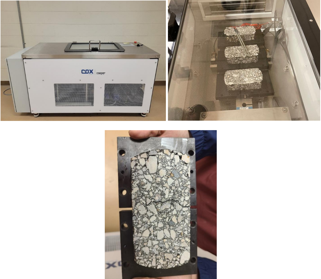
Figure 3.20. Overlay Test setup
