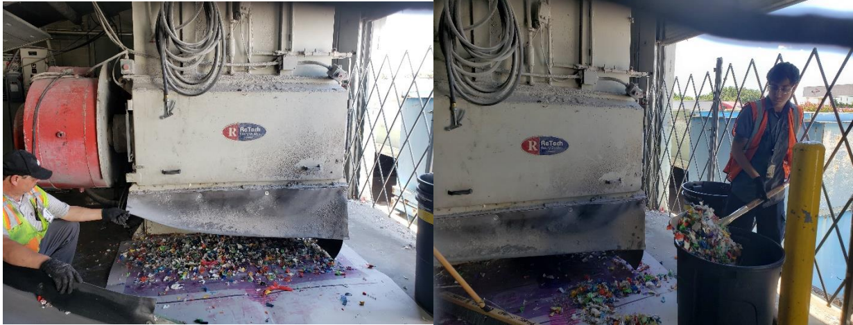
Figure 3.8. Shredding and collection of plastic
