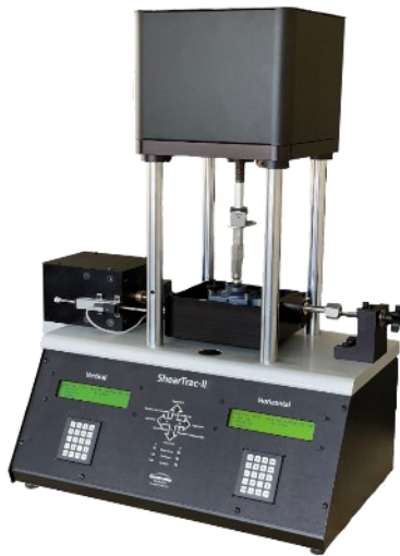
Figure 3.4 Geocomp ShearTrac-II direct shear apparatus and its specifications
