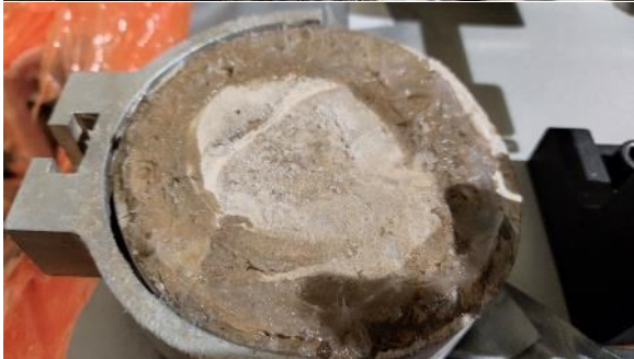
Sample ID WC1SUR04A w/c = 0.45 PAVIX Set temp 30 °F
