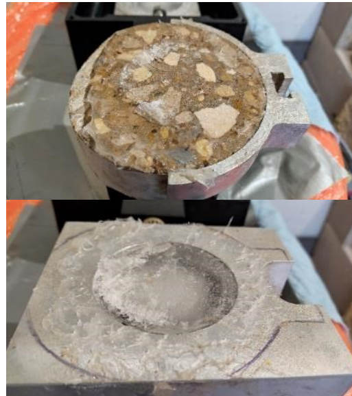
Sample ID WC1SUR04B w/c = 0.45 Control Set temp 30 °F
