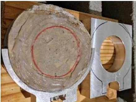
PAVIX-Treated Disk with Rough Surface
