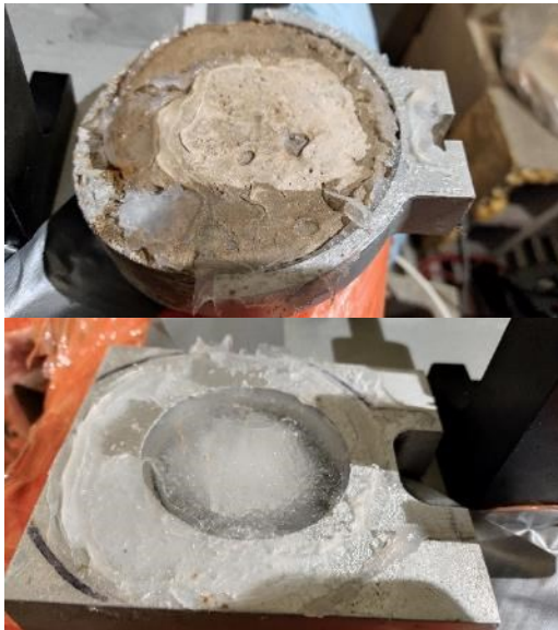
Sample ID WC1SUR05A w/c = 0.45 PAVIX Set temp 30 °F
