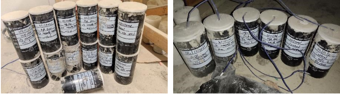
Figure 3.1 Concrete cylinders with and without Type-T thermocouple
