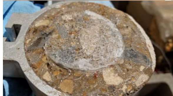
Sample ID WC1SUR04B w/c = 0.45 Control Set temp 30 °F
