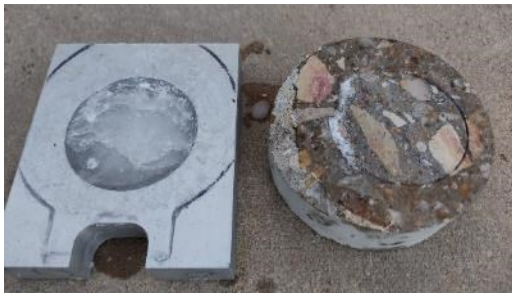
Sample ID WC1SUR03B w/c = 0.45 Control Set temp 13 °F
