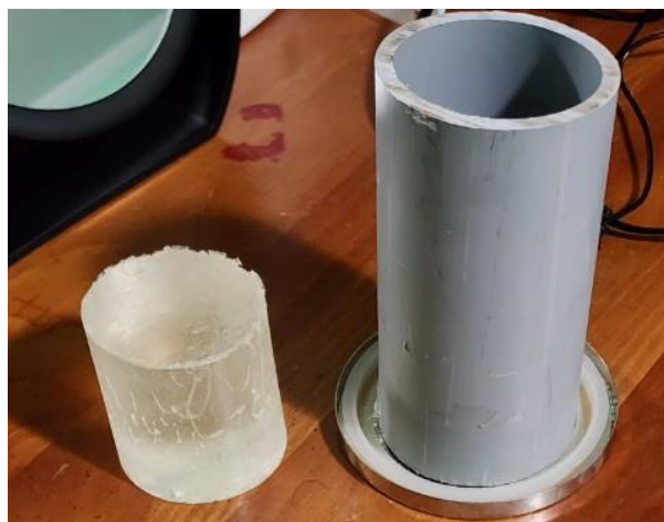
Figure 3.5: Tube Termination Cast From Epoxy
