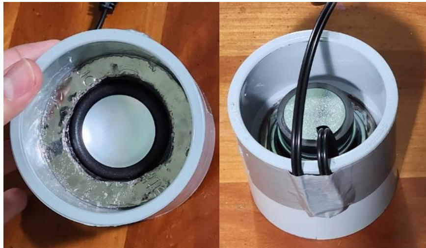
Figure 3.4: Impedance Tube Speaker End (Left:Inside, Right:Outside)
