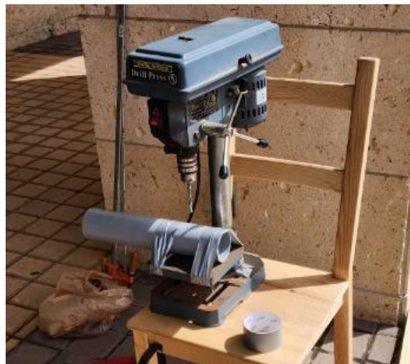
Figure 3.2: PVC Pipe Installed in Drill Press for Microphone Hole Drilling
