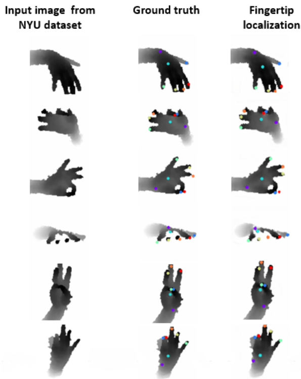
Figure 11: Qualitative results on examples of test data from NYU hand dataset; first column real depth image, second column ground truth locations and third column represents the translated image using Cycle-constituency approach
