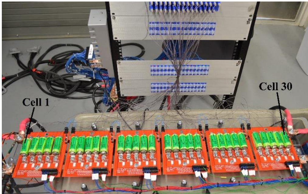
Figure 5: 1S/30P battery and thermocouple input ports
