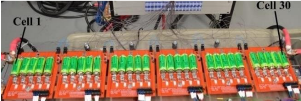
Figure 9: 1S/30P battery and thermocouple input ports
