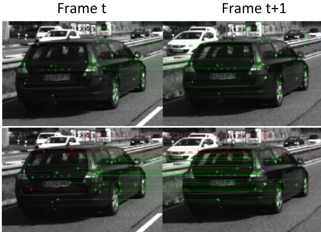
Fig. 6.8 Qualitative comparison of Deep-PT Vs. forward-backward KLT-tracker where the lines show correspondences. Top row: visualization of the tracking performed by the Deep-PT over a cropped region of an image from KITTI Flow dataset. Bottom row: visualization of the tracking performed on the same image by the KLT-tracker
