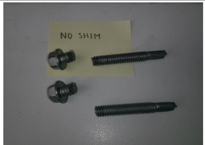
Fig V – Single shear failure
