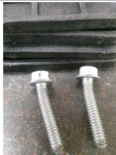
Fig. R.4 - Screws Bent
