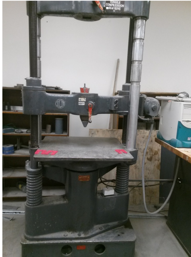
Fig. CA.2 Compression Machine with arm installed
