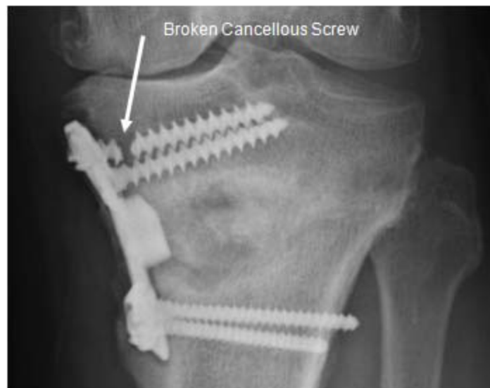
Fig. B – Surgical screw failed in Bending
