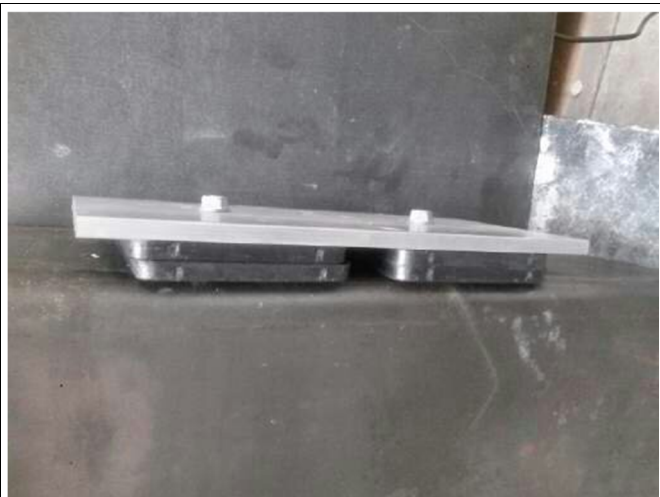
Fig. P.1 Sample Mounted (2)1/4" Horseshoe Shims
