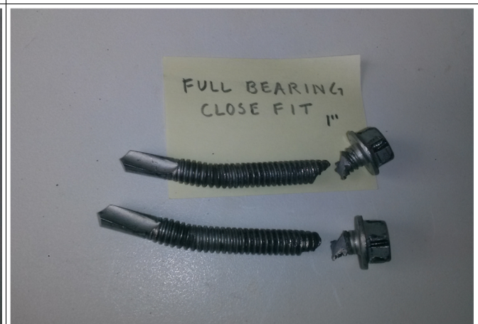
Fig O – Full Bearing Close Fit shims 1"
