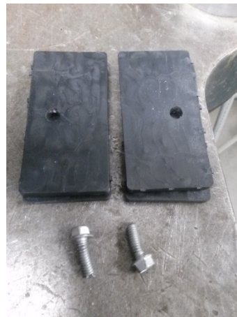
Fig. U.4 - Bent screws
