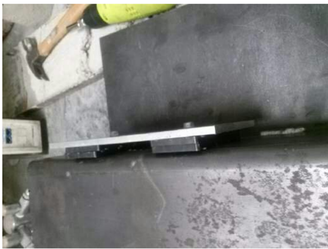
Fig. U.1 Sample Mounted (2)1/4" Full Bearing Free Fit
