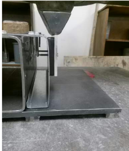
Fig T – 18 Gage Stud Mounted on Steel Tube
