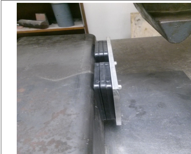
Fig. Q.1 Sample Mounted (3) 1/4" Horseshoe Shims
