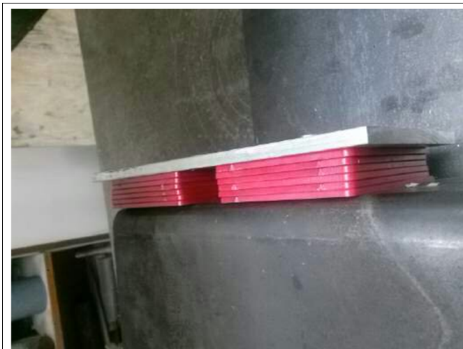
Fig. S.1 Sample Mounted (6)1/8" Horseshoe Shims
