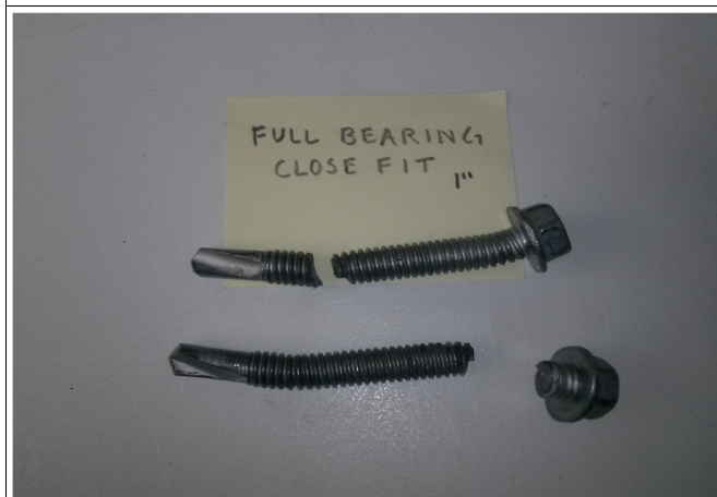
Fig N – Full Bearing Close Fit shims 1"
