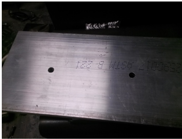
Fig. R.5 – \frac{1}{4} " Holes on Aluminum Plate
