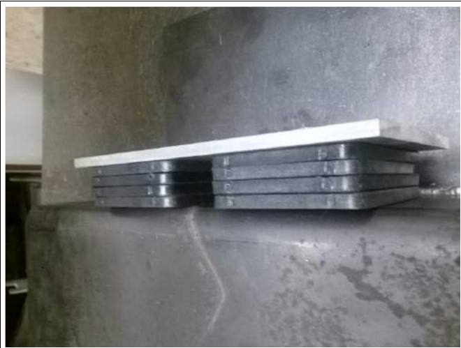
Fig. R.1 Sample Mounted (4) 1/4" Horseshoe Shims
