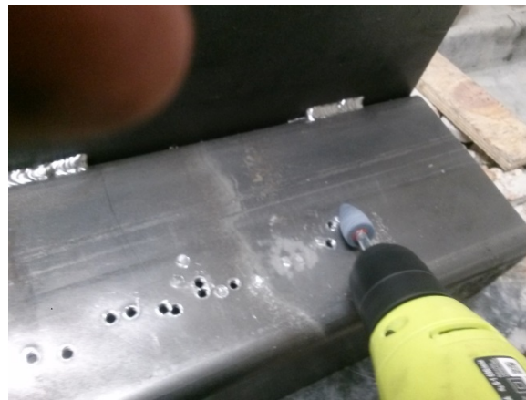
Fig. I – Restoring surface for next test
