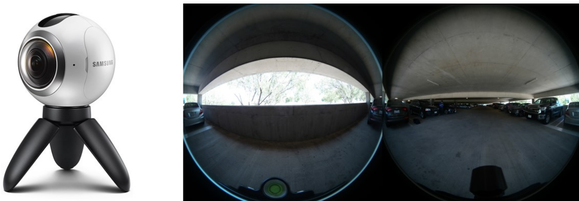
Figure 1.1: (a) Samsung Gear 360 Camera (left). (b) Gear 360 dual-fisheye output image (7776 x 3888 pixels) (right). Left half: image taken by the front lens. Right half: image taken by the rear lens.
