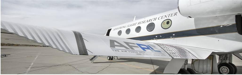
Figure 1.1: Adaptive compliant trailing edge ([www.nasa.gov](http://www.nasa.gov)).
