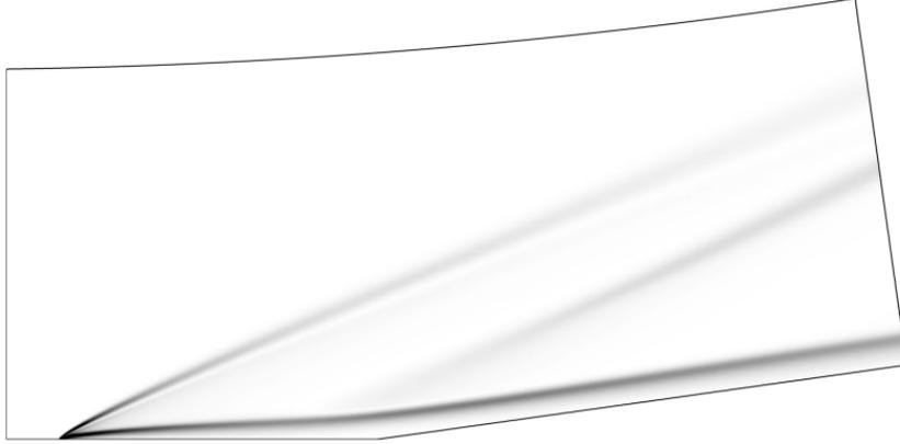
Figure 4.5: Numerical schlieren image of incipient separation conditions ( $M_\infty = 3$ ,  $\alpha = 8$  degrees,  $Re_L = 11\,232$ ).
