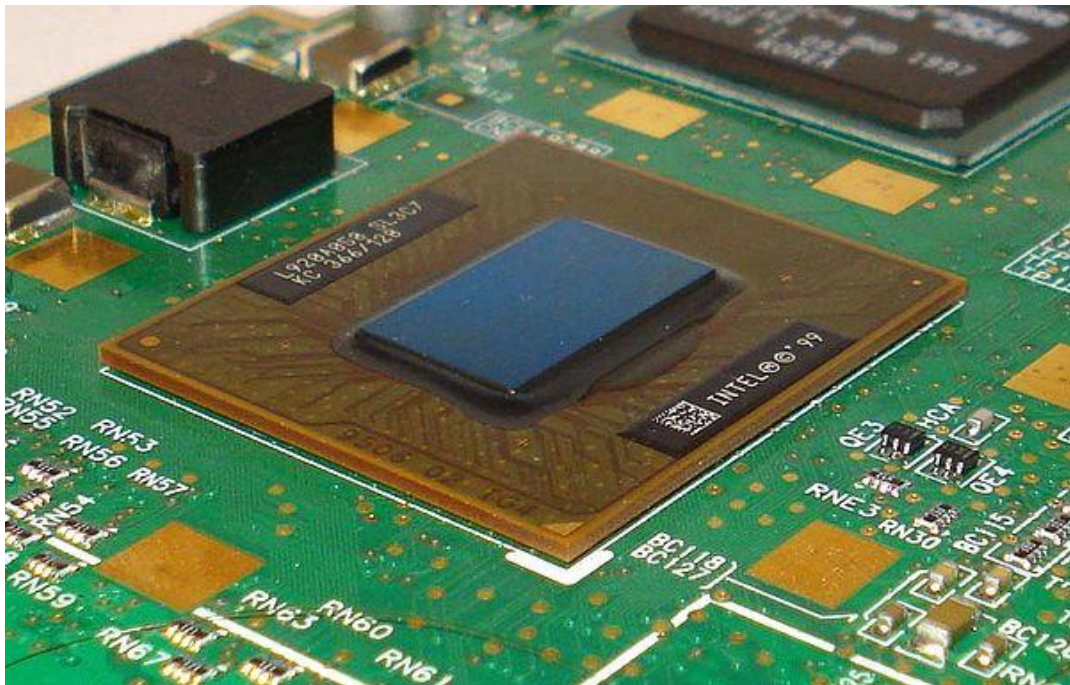
Fig: 1.4 Intel Mobile Celeron in BGA2 Package (FCBGA-479); the die is the blue
