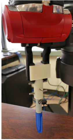
Figure 2.7. The 3D printed pen mount for the Baxter gripper.
