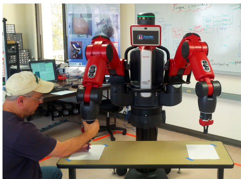
Figure 2.1. The Baxter robot being setup for a writing precision test.
