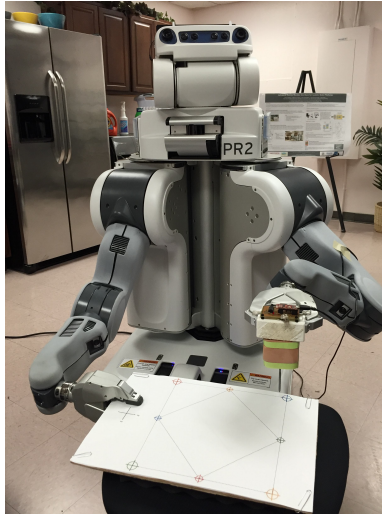
Figure 9.5. Setup for calibration and performance testing.
