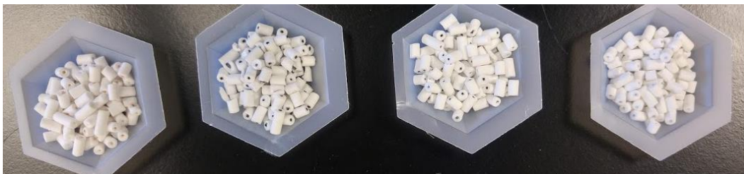
Figure 4-2 SiO 2 catalyst support with different heat conductive materials
