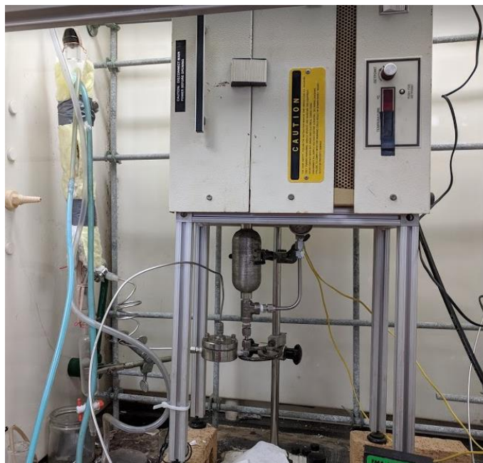
Figure 5-1 Fischer-Tropsch synthesis experimental setup with condenser unit and graduate flask liquid collector (2nd design)
