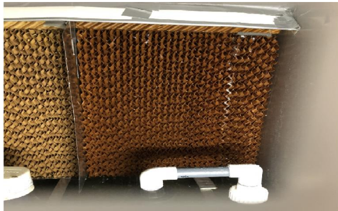
Figure 3-10 shows 66% DEC cooling media under test
