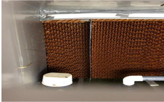
Figure 3-15 shows 100% wet DEC media under test.
