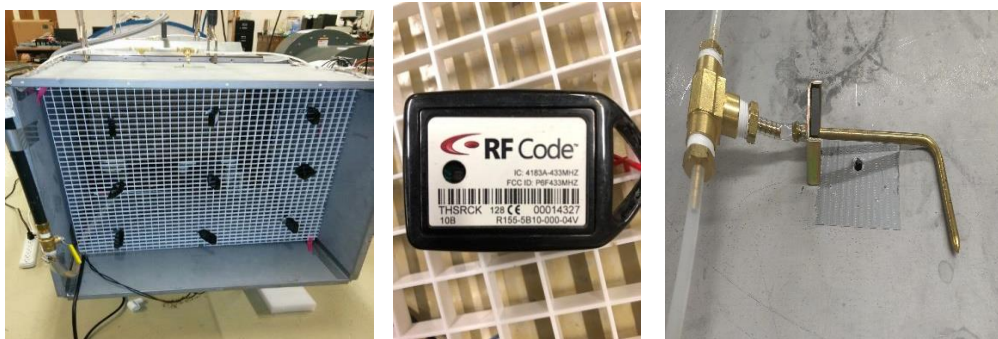
Figure 2-8 Plastic egg crate light diffusers, RF Code R155 Sensor and Dwyer A-302F-A pressure taps
