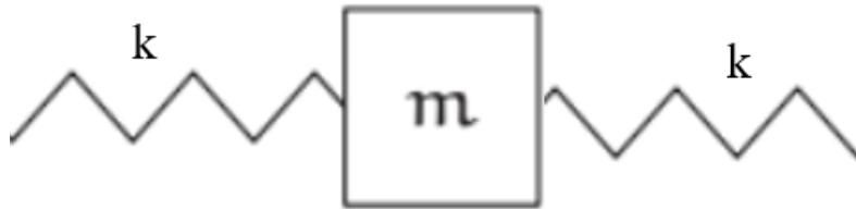
Figure 4-22: Type II unit cell equivalent spring-mass model.
