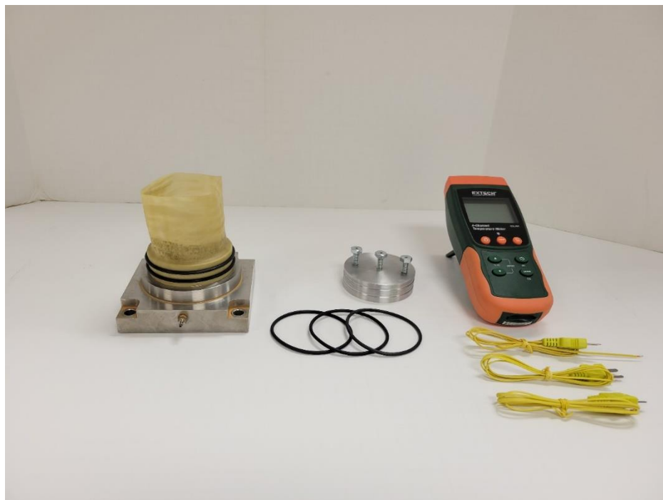
Figure 4.47: Thermo-calibration assembly step 1: secure latex membrane to base pedestal using 2 rubber O-rings and add soil sample.
