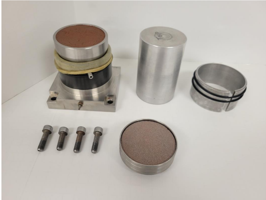
Figure 4.19: Sample pedestal assembly step 4: place the sample ring with the remolded soil sample onto the sample former.
