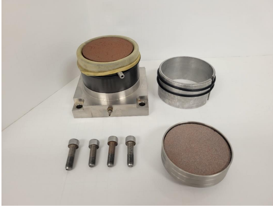
Figure 4.21: Sample pedestal assembly step 6: remove solid aluminum compaction cylinder and sample ring from the sample pedestal.
