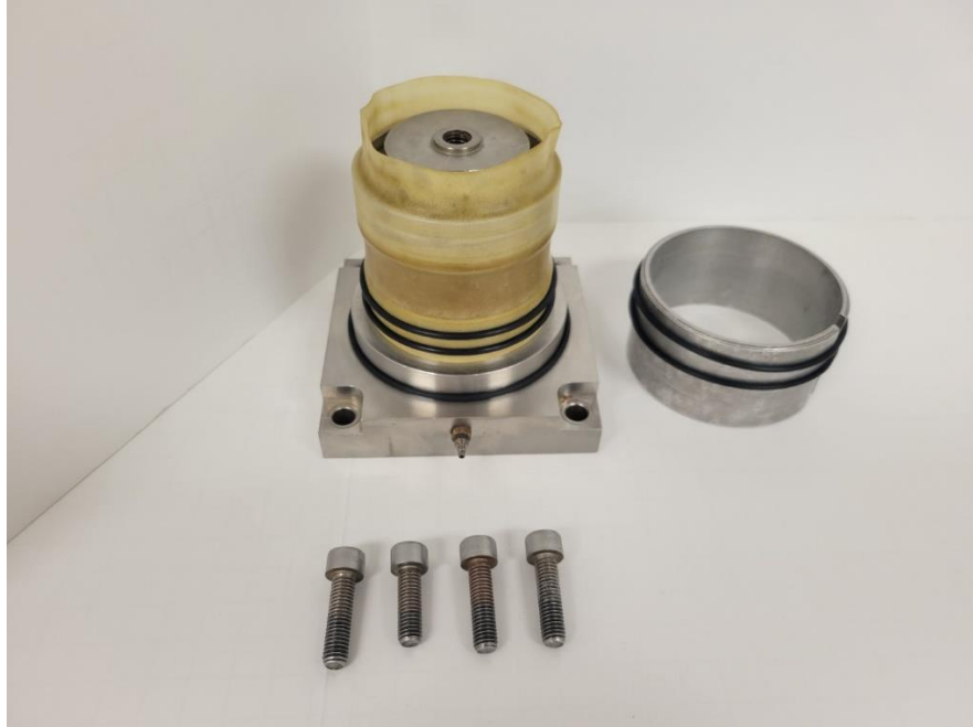
Figure 4.23: Sample pedestal assembly step 8: pull latex membrane over top cap and remove sample former. To remove sample former, roll rubber O-Ring down off of the sample former and onto the base plate as shown. May need to carefully adjust membrane and top cap to ensure membrane is pulled tight with no creases or folds.
