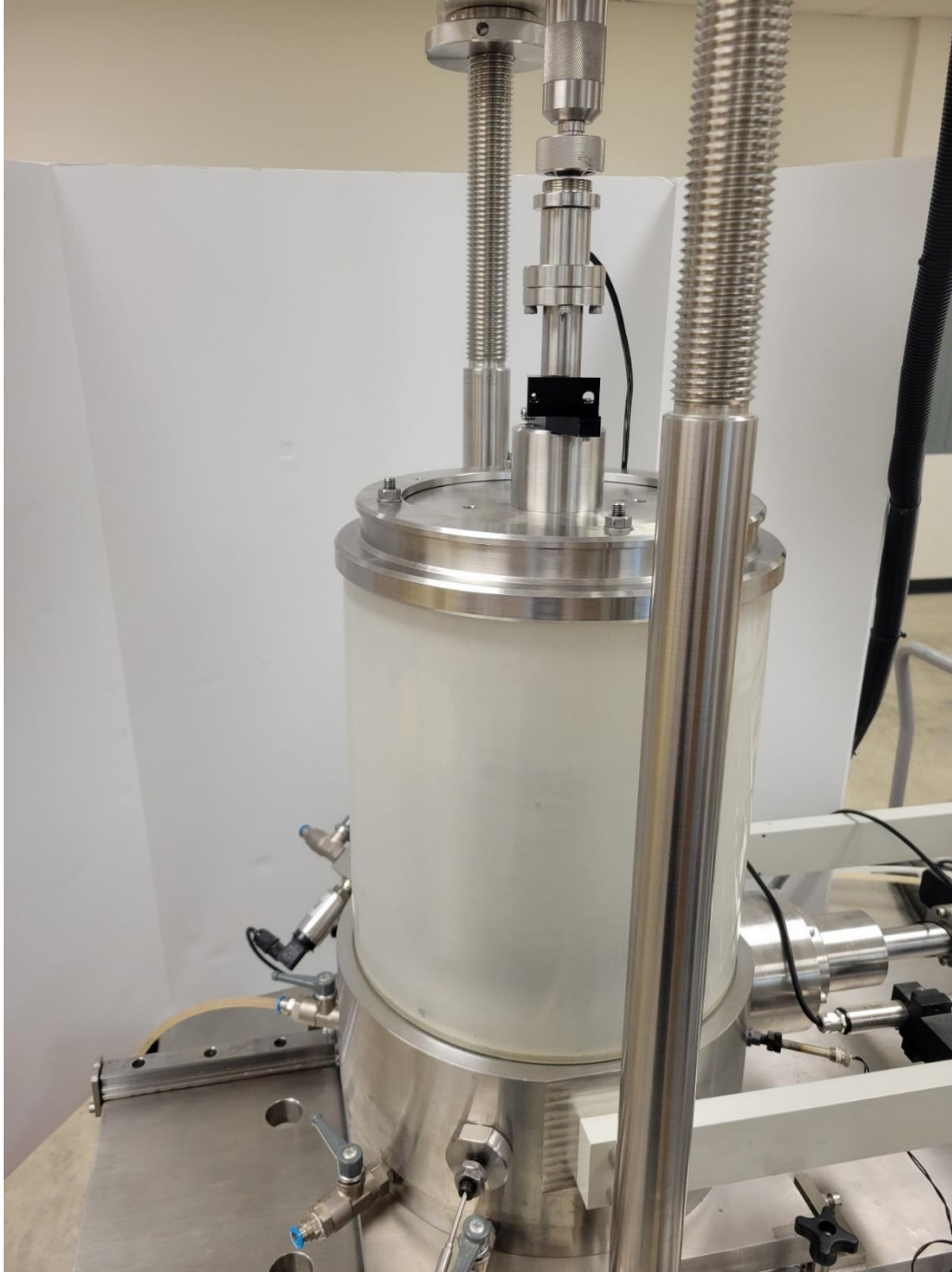
Figure 4.37: Confining cell assembly step 13: push the cell back into position under the cross beam of the vertical servo.
