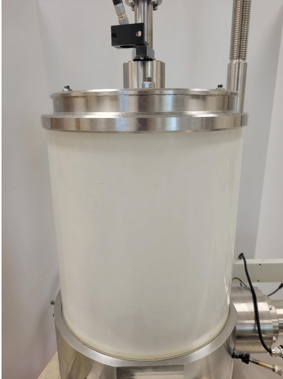
Figure 4.36: Confining cell assembly step 12: place the cell top onto the cell wall such that the 4 screw heads on the cell body come out of the 4 holes in the cell top. Push down on the cell top until it drops down into a secure position. Place a washer and nut on each screw head and cross tighten to seal the top cap.
