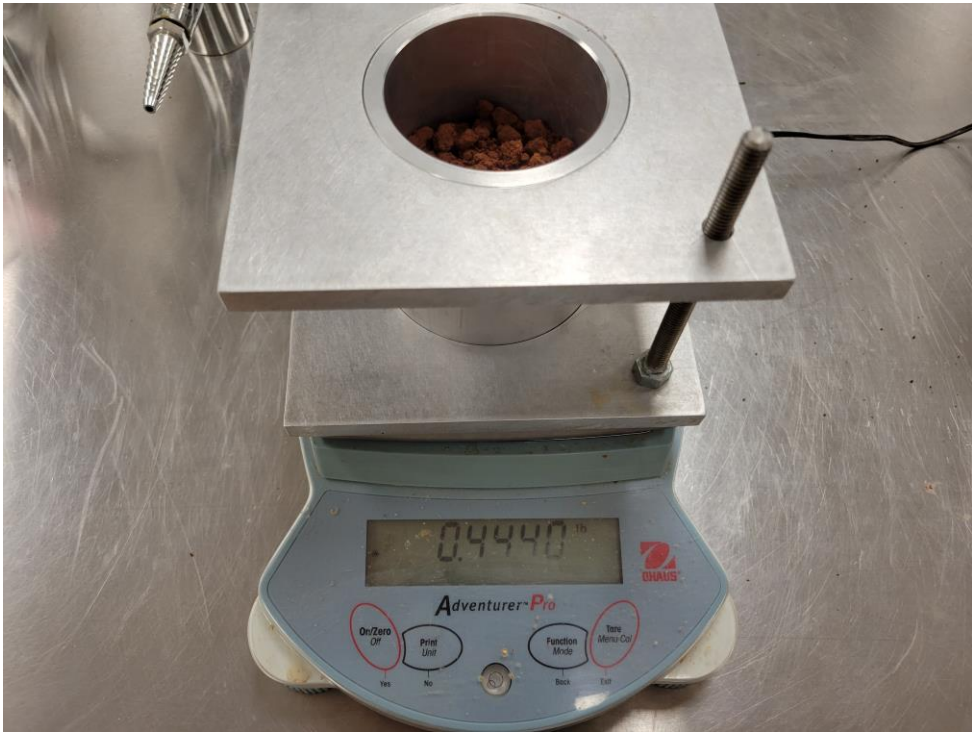
Figure 4.9: Fill mold with calculated amount of soil to achieve desired dry density after compaction.
