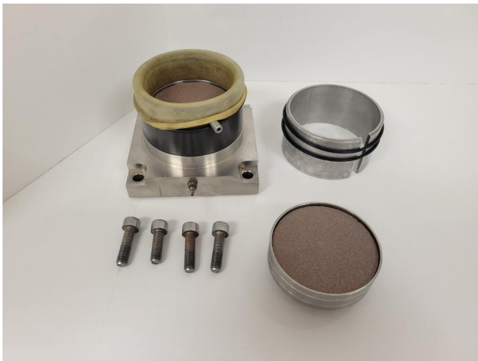
Figure 4.18: Sample pedestal assembly step 3: place the sample former over the membrane onto the base pedestal, fold the top of the membrane over the sample former as shown.
