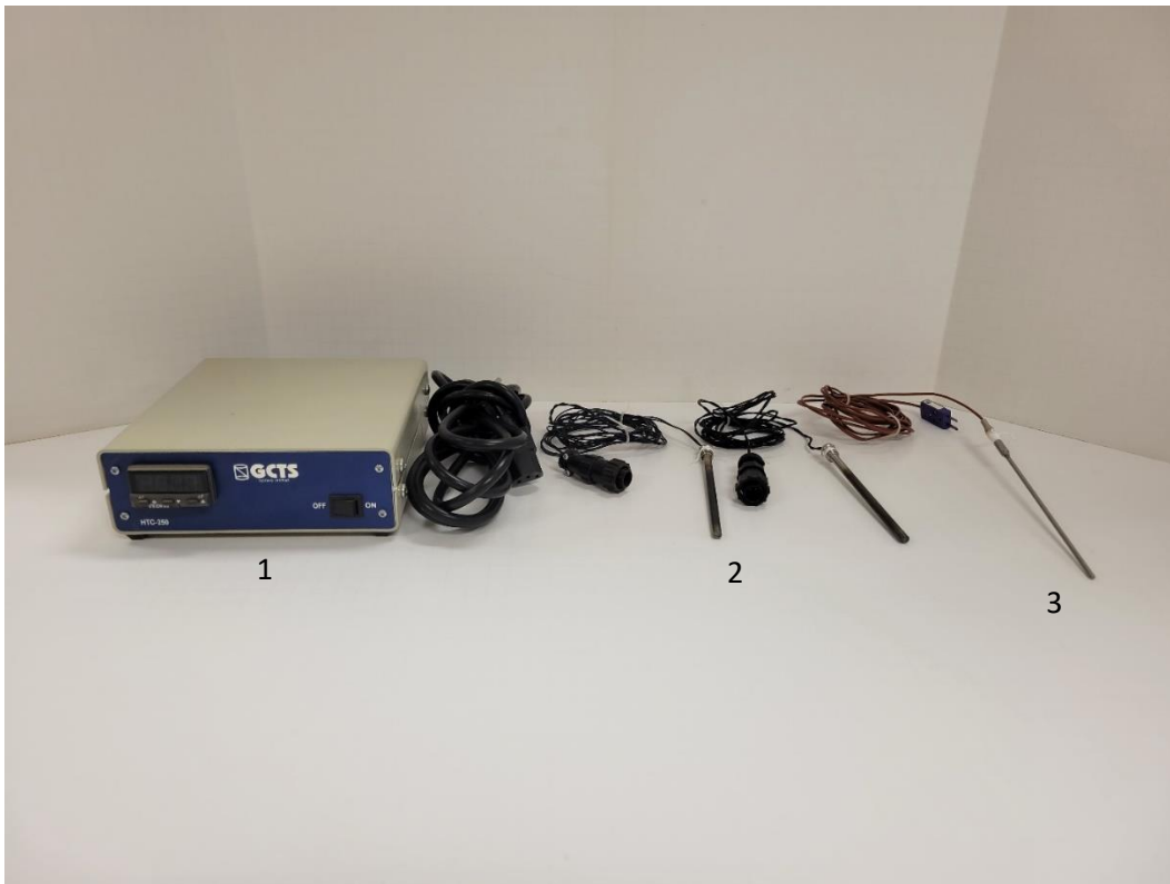
Figure 4.43: GCTS HTC-250 Heater Control Unit components: 1) control box, 2) 2 heating elements, 3) thermocouple
