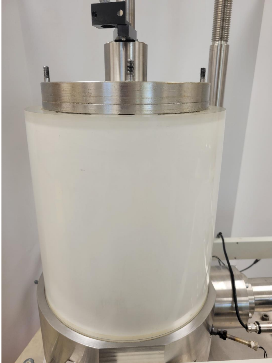
Figure 4.35: Confining cell assembly step 11: place the cell wall over the cell base. Make sure the cell wall is seated centrally on the base.
