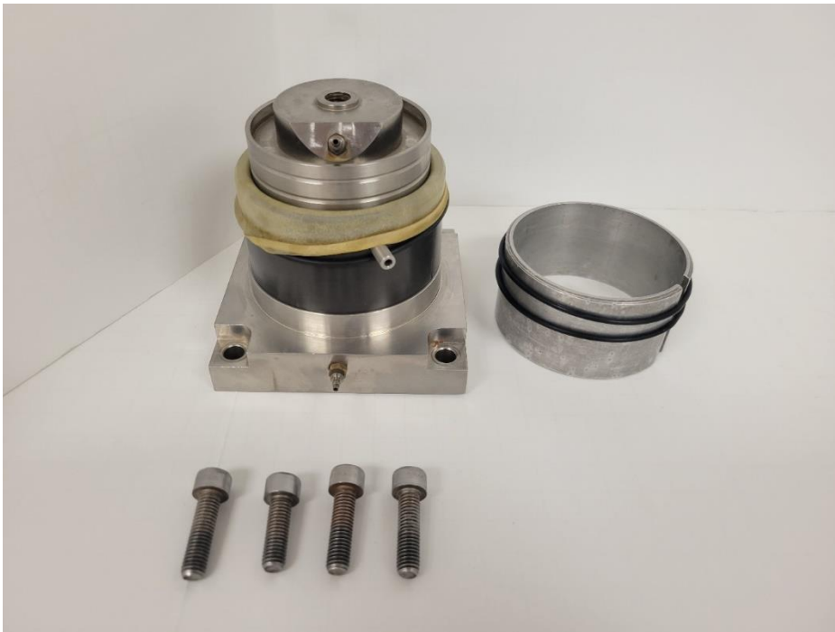
Figure 4.22: Sample pedestal assembly step 7: place top cap onto sample former and press down lightly to seat top cap onto sample. Take care to ensure that the valve on the base plate is pointing the same direction as the valve on the top cap for easy assembly.
