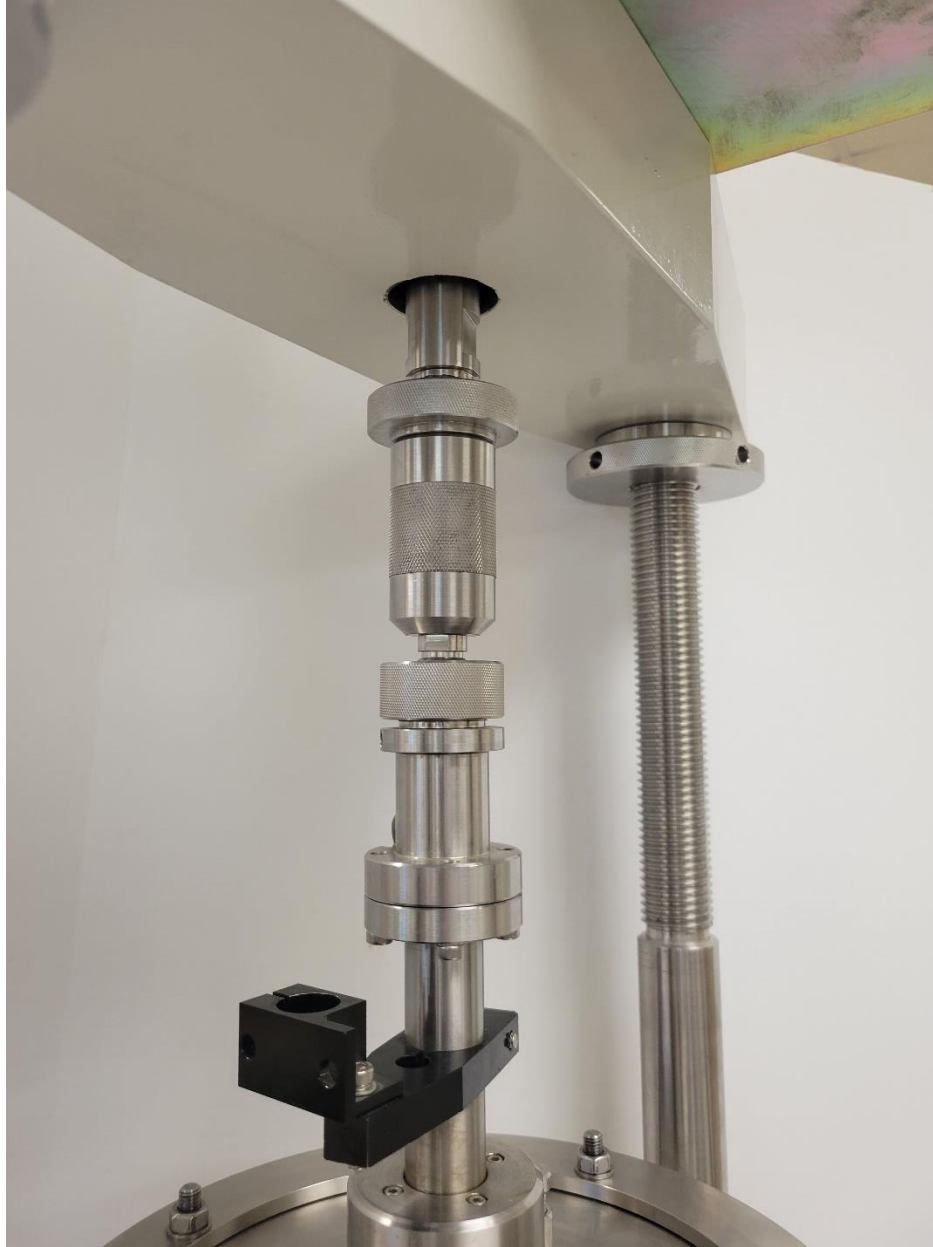
Figure 4.39: Confining cell assembly step 15: connect the vertical ram to the vertical servo. Adjust the adapter until the ball and cup joint are touching then use the milled nut to secure the vertical ram similar to the process followed for the horizontal ram. Do not apply load to the sample. Loosen the top bracket and move into a neutral position.
