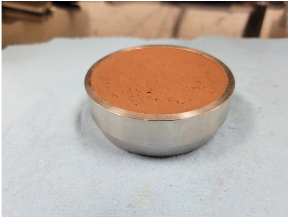
Figure 4.11: Disassemble compaction mold to reveal steel ring with compacted soil sample.
