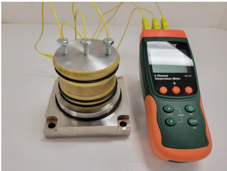
Figure 4.49: Thermo-calibration assembly step 3: insert three wire probes into soil sample using the corresponding three holes in the top cap.
