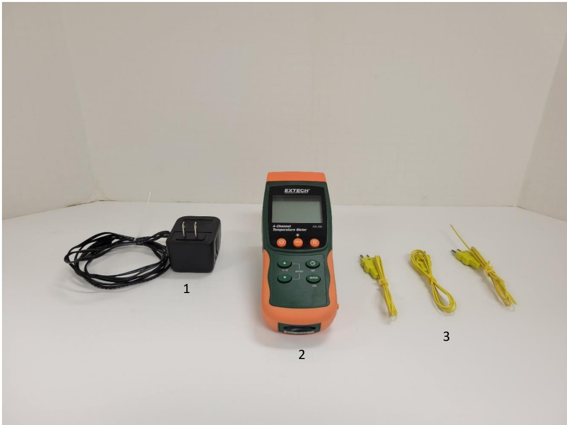
Figure 4.45: Extech 4-Channel Data Logging Thermometer components: 1) power cable, 2) thermometer, 3) 3 thermocouple wire probes
