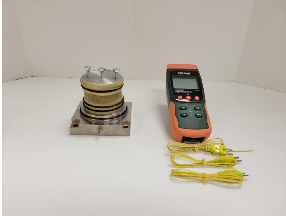
Figure 4.48: Thermo-calibration assembly step 2: firmly place top cap onto soil sample and secure latex membrane to top cap using 2 rubber O-rings.
