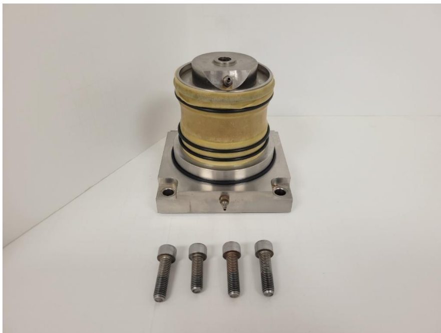
Figure 4.24: Sample pedestal assembly step 9: Use the O-Ring tool to place the last 2 rubber O-Rings onto the latex membrane and into the grooves in the top cap, firmly securing the membrane to the top cap. Fold the membrane down to expose the valve in the top cap.
