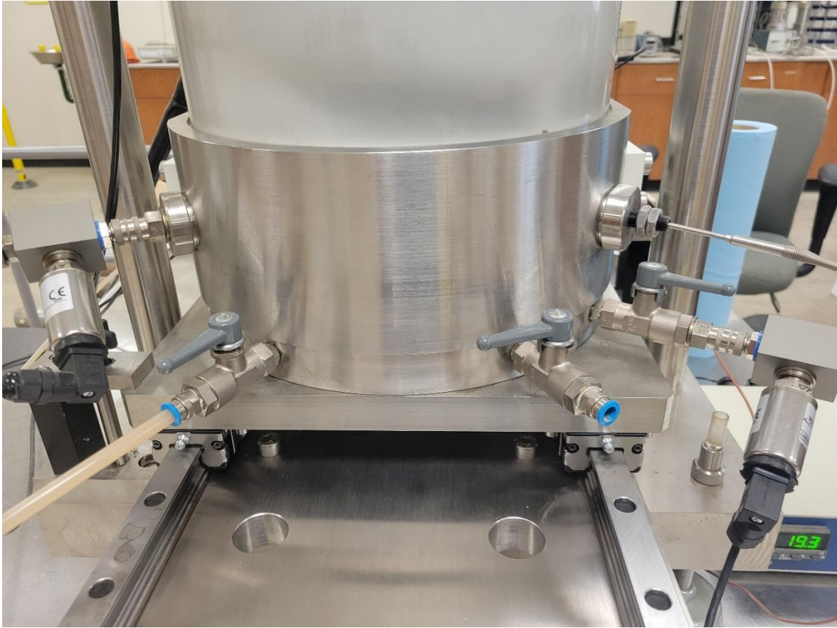
Figure 4.42: Confining cell assembly step 18: connect cell pressure line from Pro Dual APC to cell pressure valve. The sample is now ready for testing.
