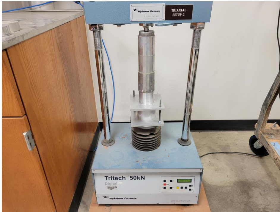
Figure 4.10: Place solid aluminum cylinder into the mold and place mold into the compaction device.
