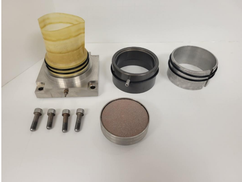
Figure 4.17: Sample pedestal assembly step 2: place standard latex membrane on base pedestal and use O-Ring tool to place 2 rubber O-Rings over the membrane and into the grooves in the base pedestal, firmly securing the membrane to the base.
