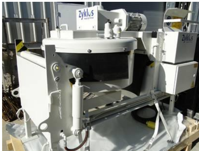
Figure 3-10 Pan mixer used for mixing UHPC specimens
