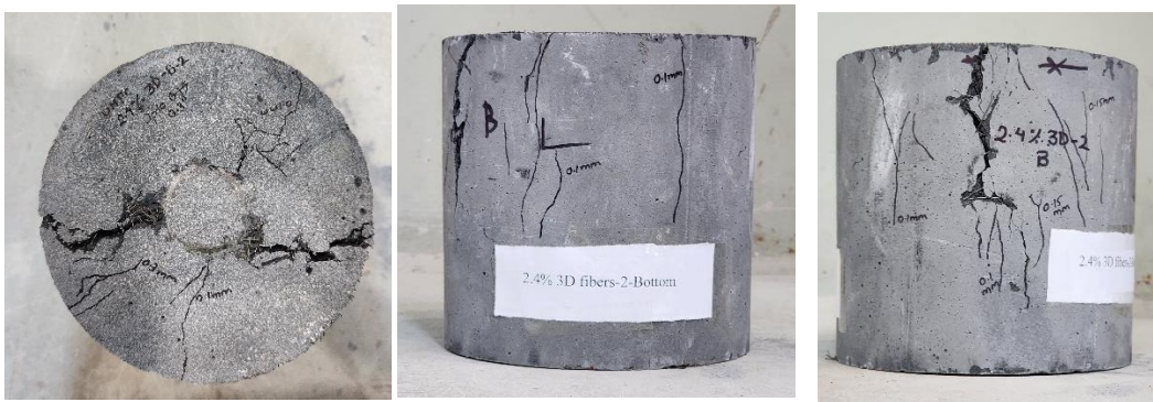
Figure 4-14 Sample DPT specimen showing cracks.
