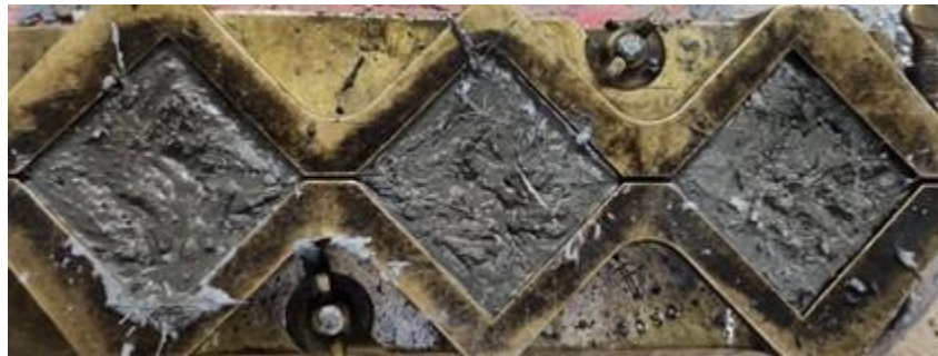
Figure 4-4 Casting of 2 in. cubes.
