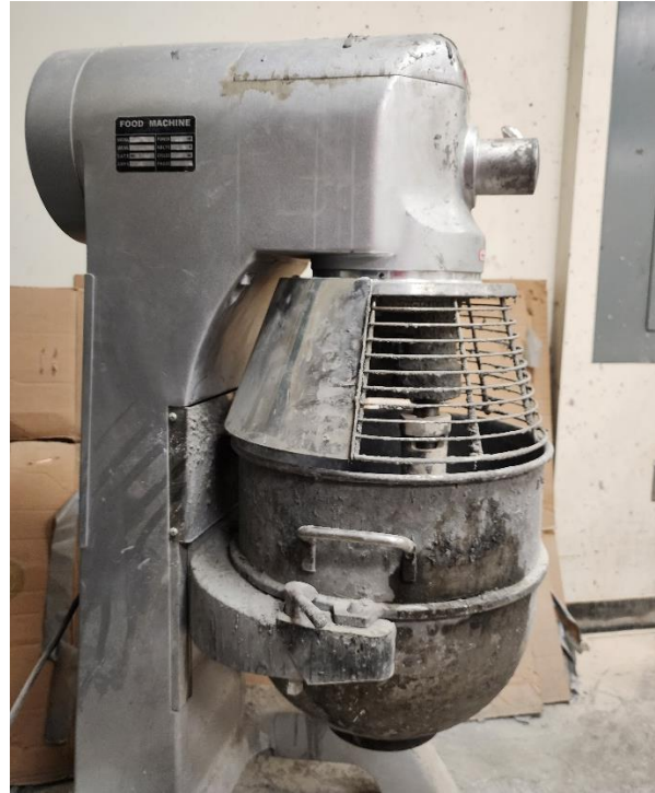
Figure 3-3 This lab mixer was used to prepare 40 quarts of UHPC.
