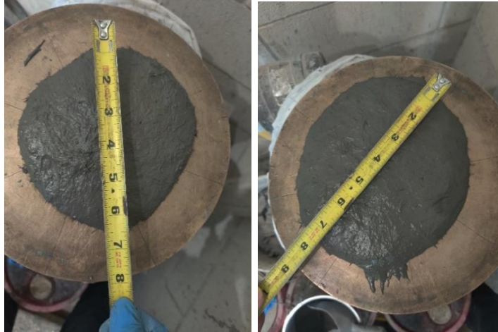
Figure 4-5 Flowability test a. 970U (w/o fly ash) b. 970U (w fly ash)
