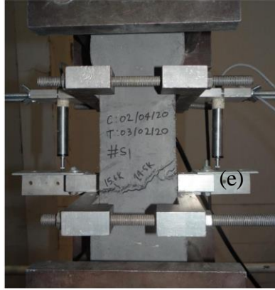
Figure 4-11 Failure for dog bone samples for straight fibers, a.1.5%, b.2%, c.2.25%, d. 2.4%, e.
