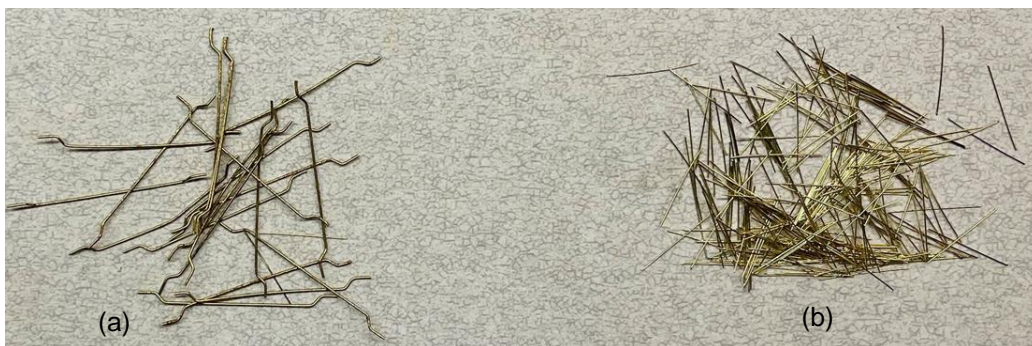
Figure 3-1 Types of fibers used in the study. (a) Hooked fibers and (b) straight microfibers
