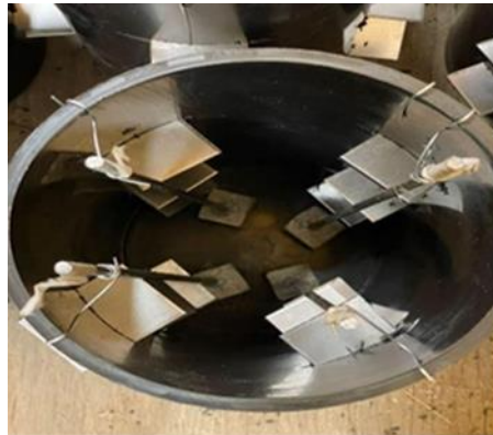
Figure 42. Placing the Wires in Cylinders
