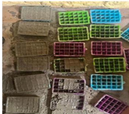
Figure 41. Concrete Cubes for Cover
