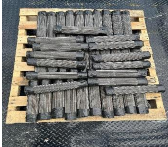
Figure 32. Wires for 24 inches of Pipe
