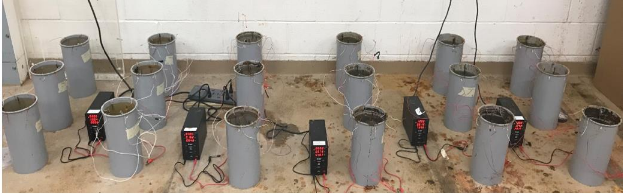
Figure 6. Accelerated Corrosion Test on Rebars
