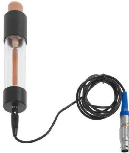
Figure 26. Rod Corrosion Electrode
