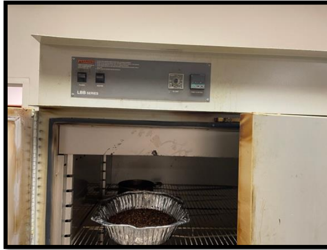
Figure 3-4 Aggregates Inside of Oven
