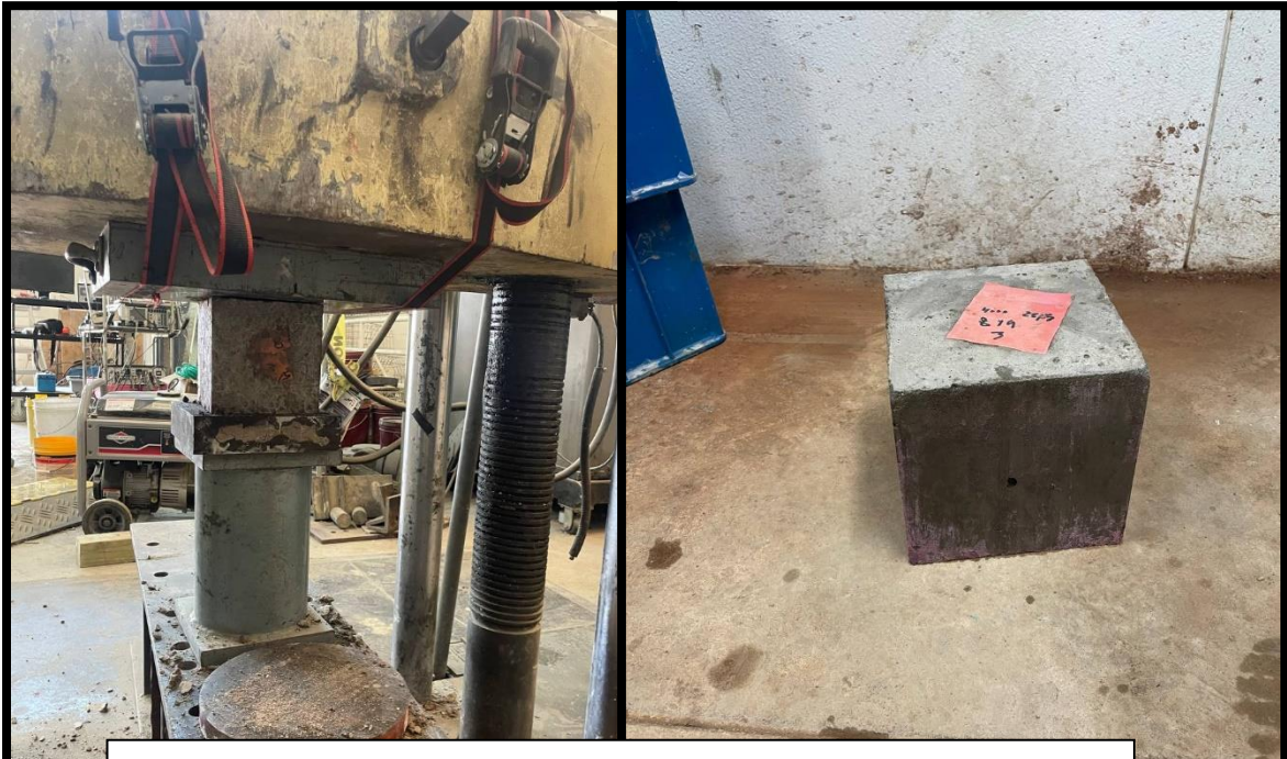
Concrete Samples Undergoing Compressive Strength Testing.
