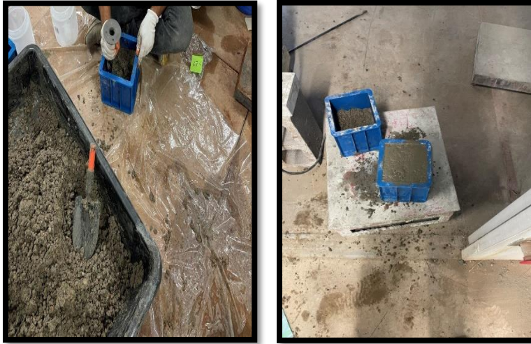
Figure 3-5 Rodding Method and Vibration Table Shaker
