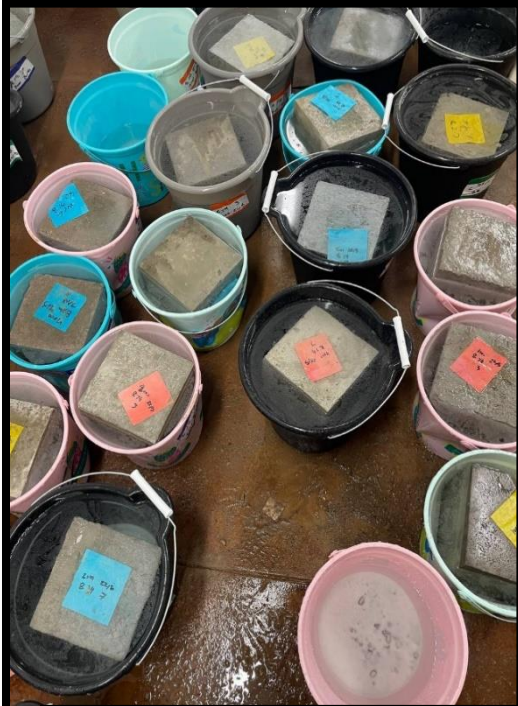
Concrete Samples Immersed in Water for Curing
