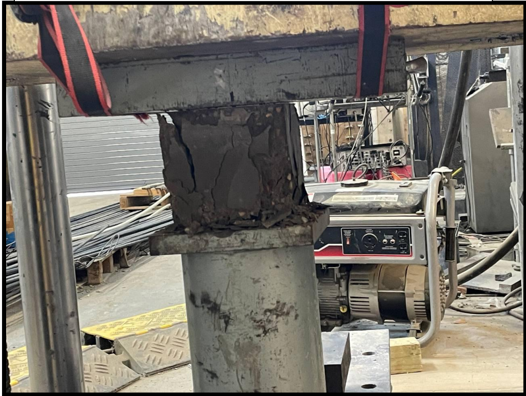
Concrete Samples Undergoing Compressive Strength Testing.
