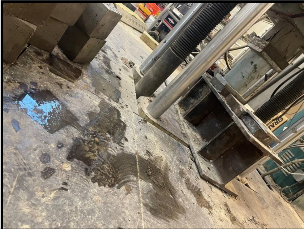
Concrete Samples Undergoing Compressive Strength Testing.
