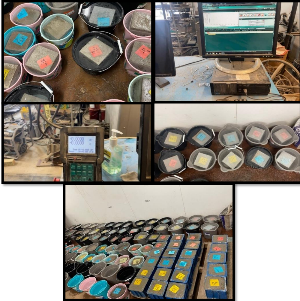
Figure 3-12 Concrete Samples Immersed in Water for Curing
