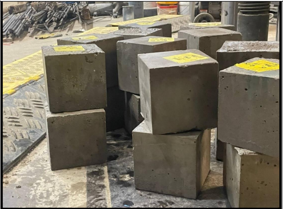
Concrete Samples Undergoing Compressive Strength Testing.
