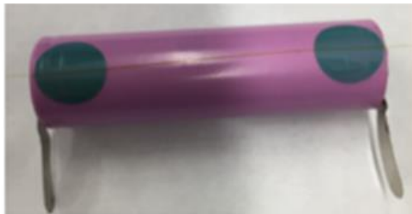
Figure 2.6. Experimental Setup Showing the Fiber Optic Sensor Taped Axially Down the Length of the 18650 Cell Under Test. ODiSI-B System Not Shown.
