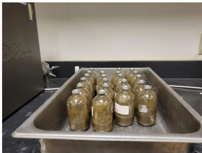
Figure 3-17: Batch reactors with rice straw
