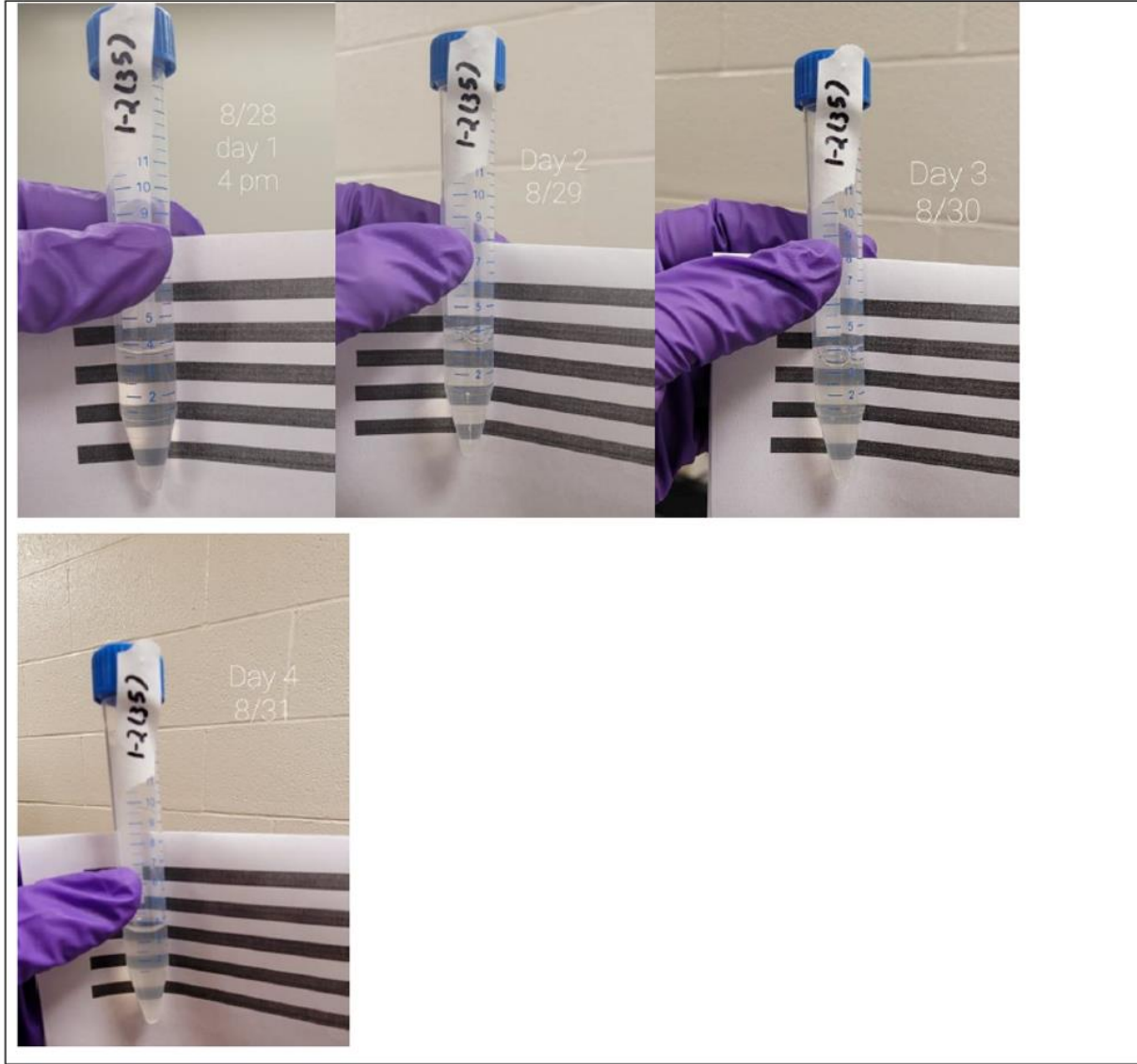
Figure 4-3: Testing Turbidity of TAV5 vs high contrast background
