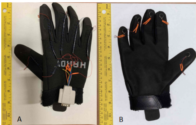
FIGURE 8: HAPTIC FEEDBACK GLOVE: A) GLOVE OUTER SIDE, B) GLOVE INNER SIDE [30]
