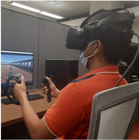
Figure 3: The human operator uses a VR headset and controllers to control the robot in a simulated in-doors environment.
