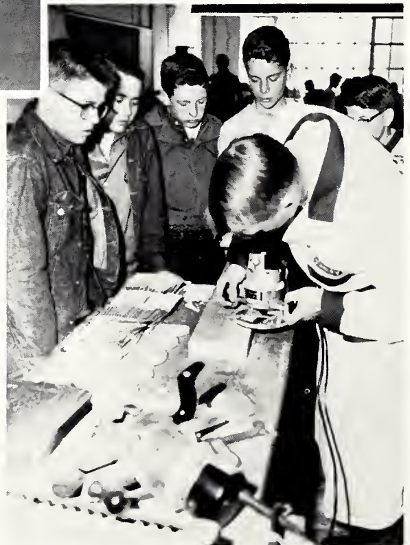
This woodshop student cuts names into a block of wood with a router.
