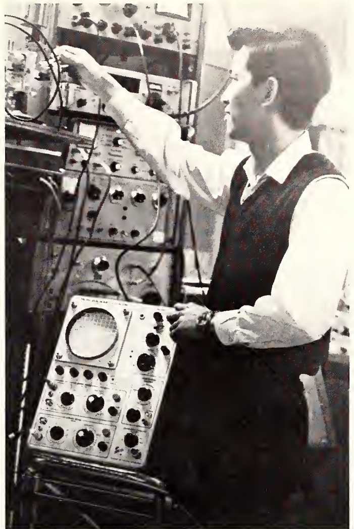
Allen Ma, a physics graduate student, calibrates the electron-spin resonance spectrometer which measures magnetic absorption in various materials.
