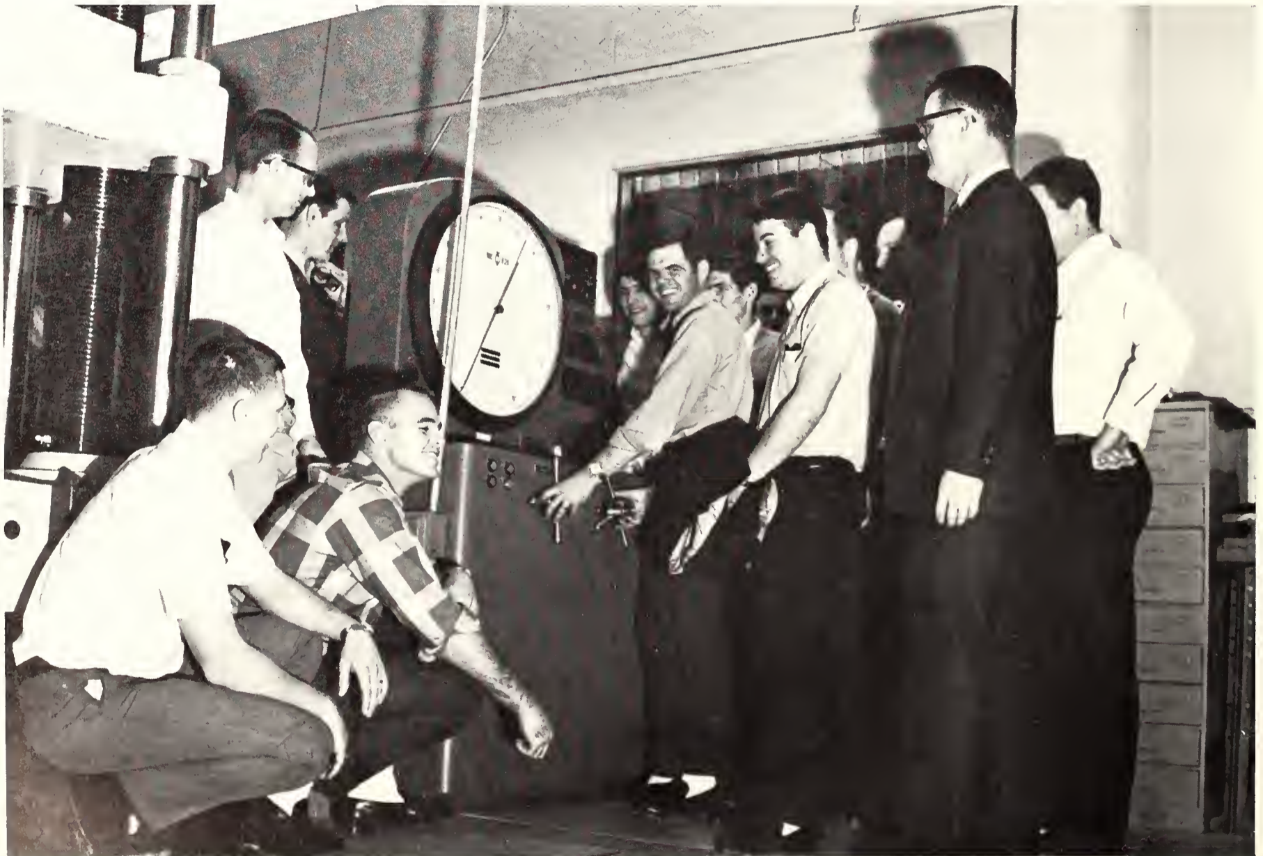
Dr. Richard Haynes, civil engineering instructor, supervises students' experimenting with a tensile and compressive test machine.
