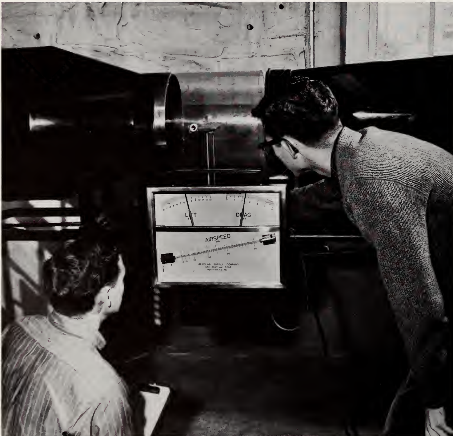
Two aerospace students make use of the department's wind tunnel to study the effects of lift and drag on the airspeed of a plane.
