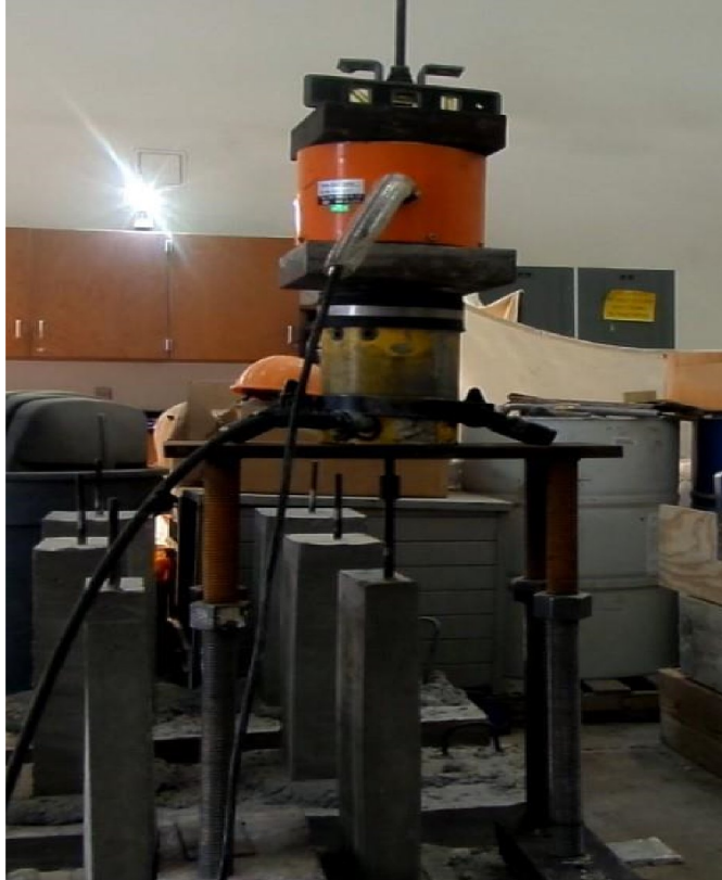
Figure 3.30 Single Anchor Pullout Test Set-Up (Lab)
