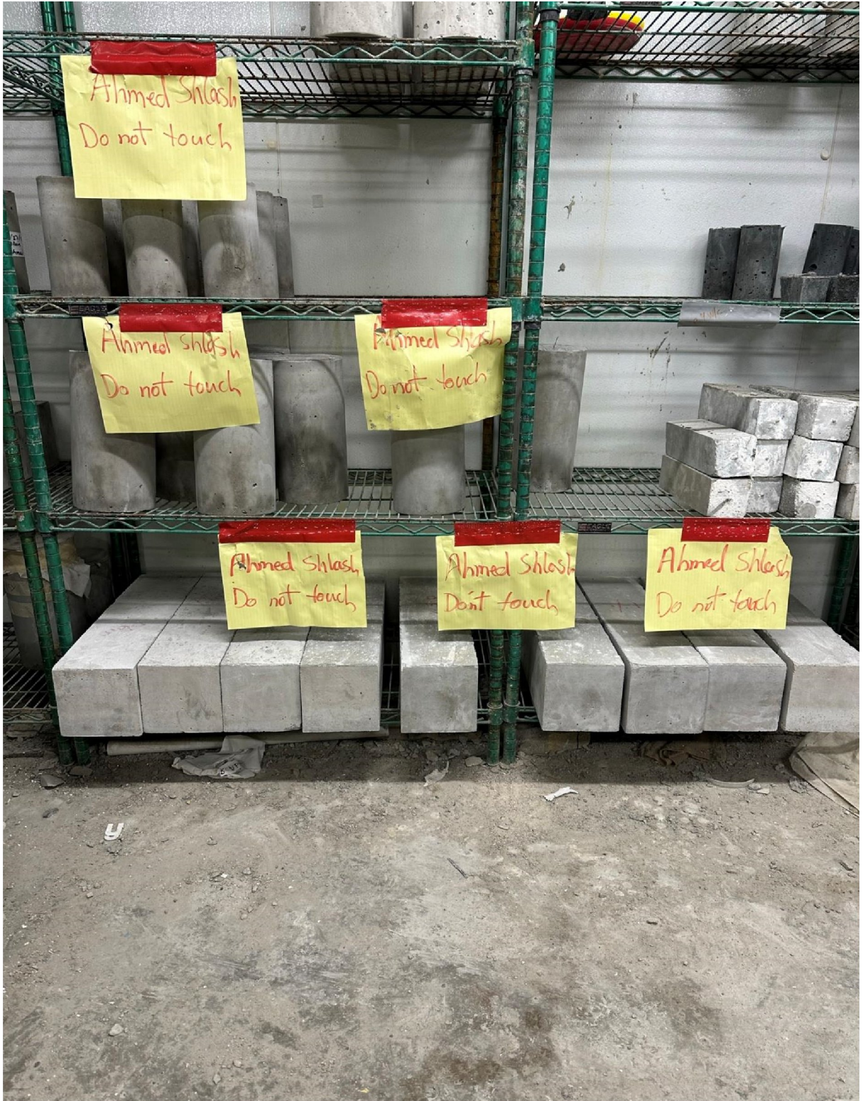
Figure 3.21 Concrete Specimens in the Curing Room
