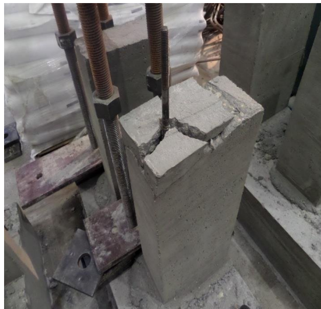
Figure 3.33 Concrete Breakout Failures (0.0% SFRC)
