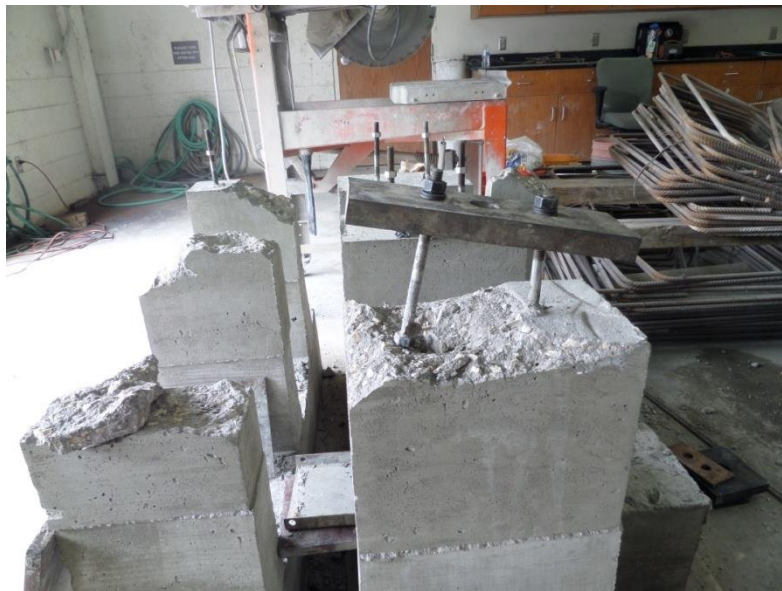
Figure 3.40 Concrete Breakout Failures (0.0% SFRC)
