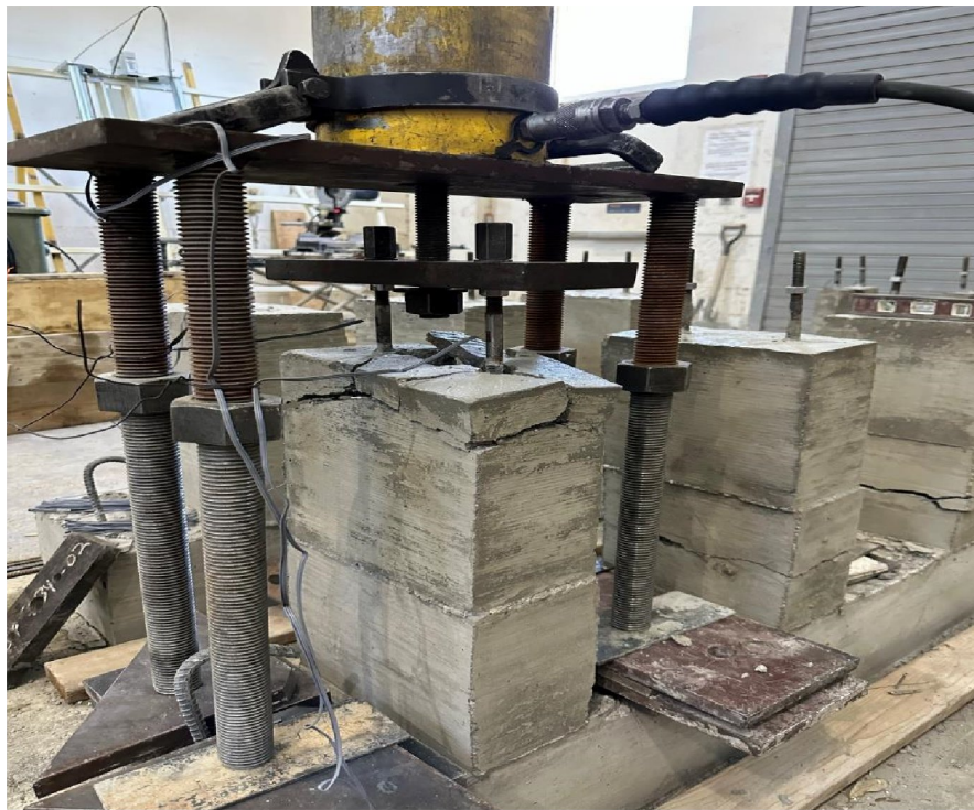
Figure 3.41 Concrete Breakout Failures (0.5% SFRC)
