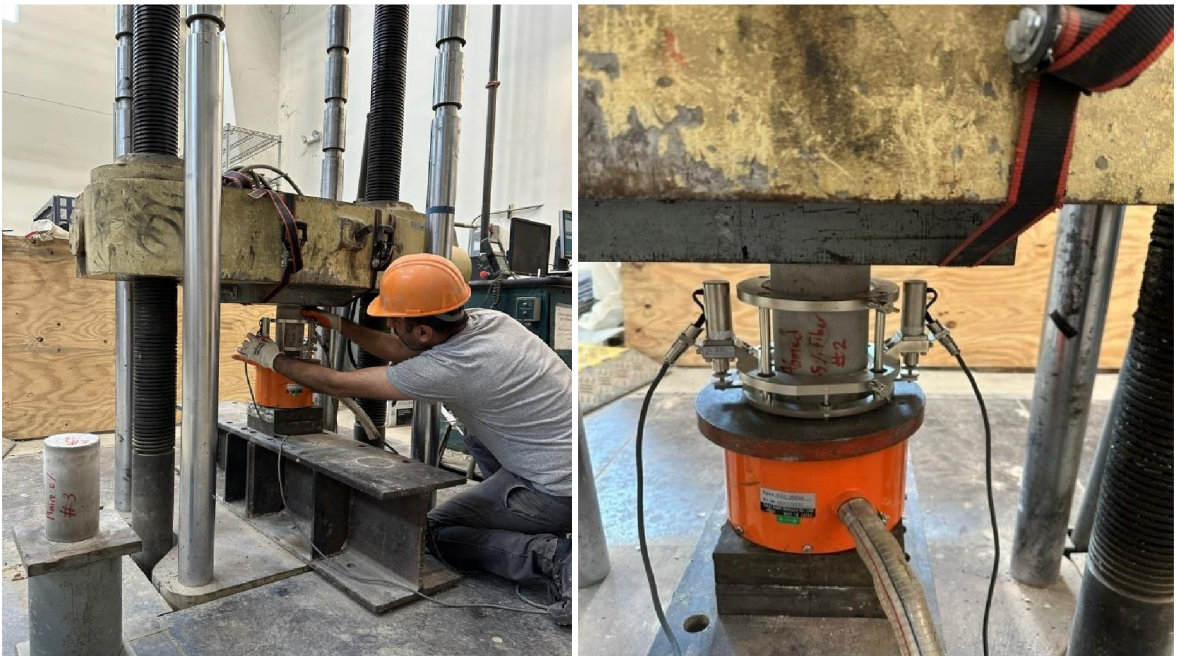
Figure 3.22 Compression Test Set-Up
