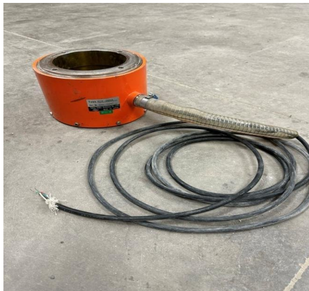
Figure 3.31 Load Cell (500KN-2MN)
