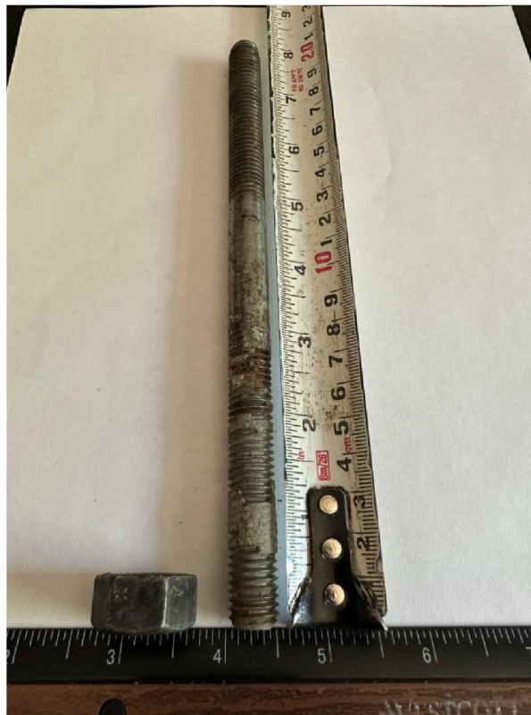
Figure 3.28 Steel Headed Stud (F1554 G105)
