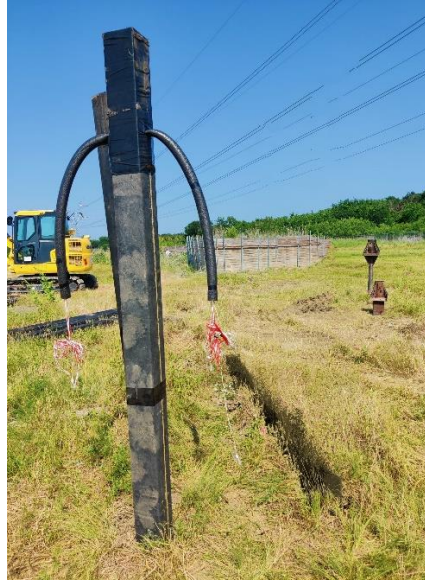
Figure 3-4 (a) Schematic Diagram of Instrumented RPPs; (b) Instrumented RPP; (c) Pressure plate
