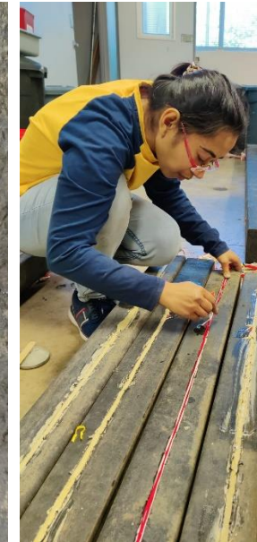
(g) Placement of wire inside the groove
