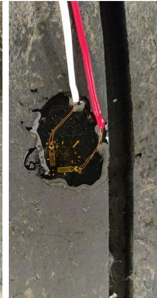
(f) Putting protective layer on the gauges
