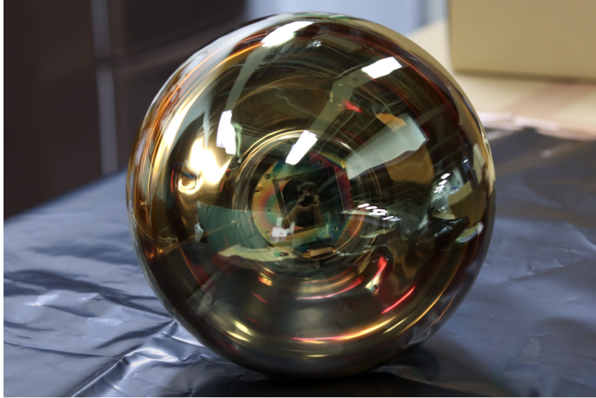
FIGURE 3.1.2: A D-Egg PMT
