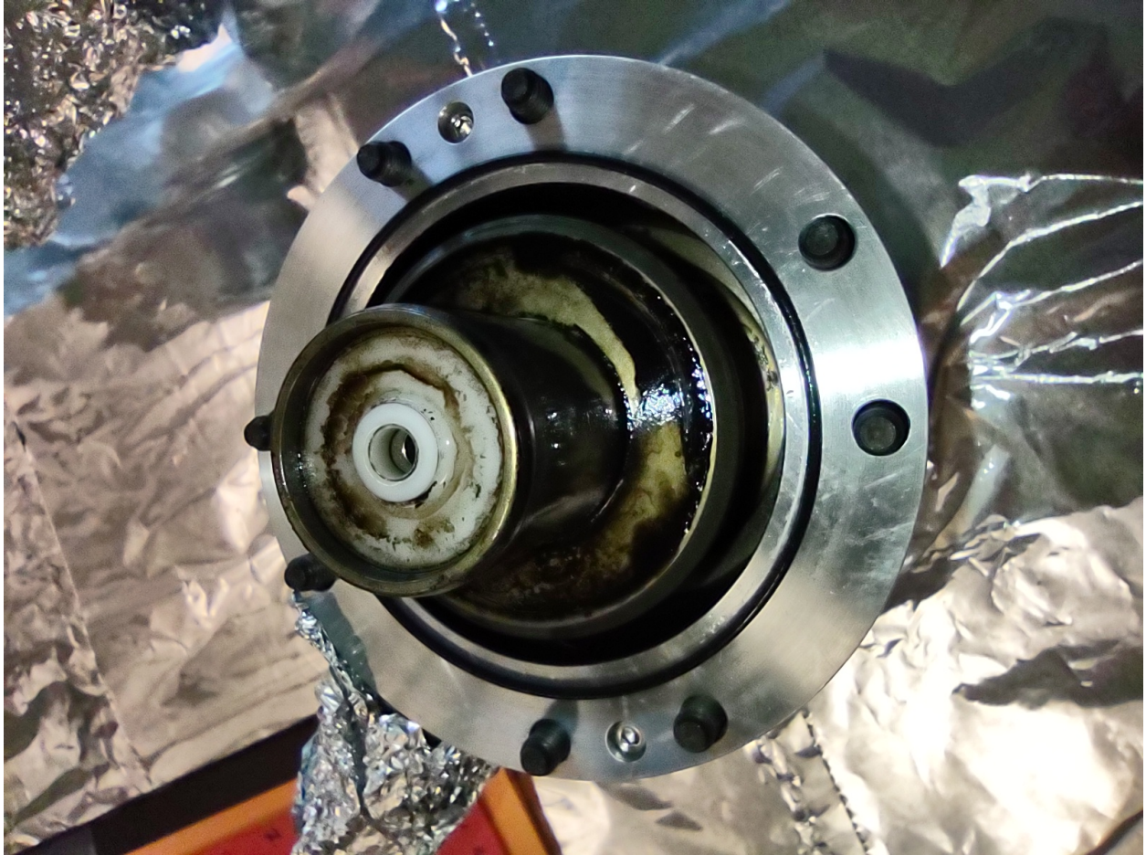
Figure 3.1: Valve motor assembly filled with oil, indicating failure of the helium compressor's adsorber.
