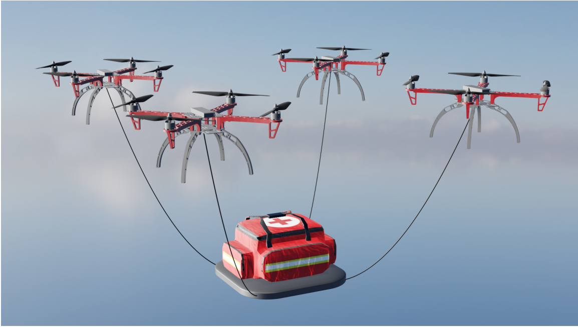
Figure 1.1: Illustration of an aerial payload manipulation mission by cooperative multi-rotors carrying an emergency bag suspended via cables
