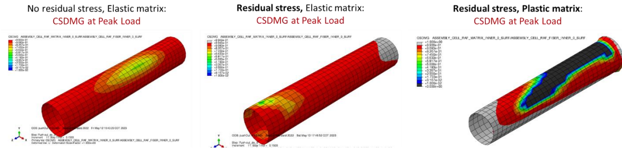
Figure 60. Interface damage at Peak Load. The combined effects of residual stress and plastic matrix damage. CSDMG > 0.99 (near total failure): colored gray; CSDMG < 0.01 (almost intact interface): colored black.
