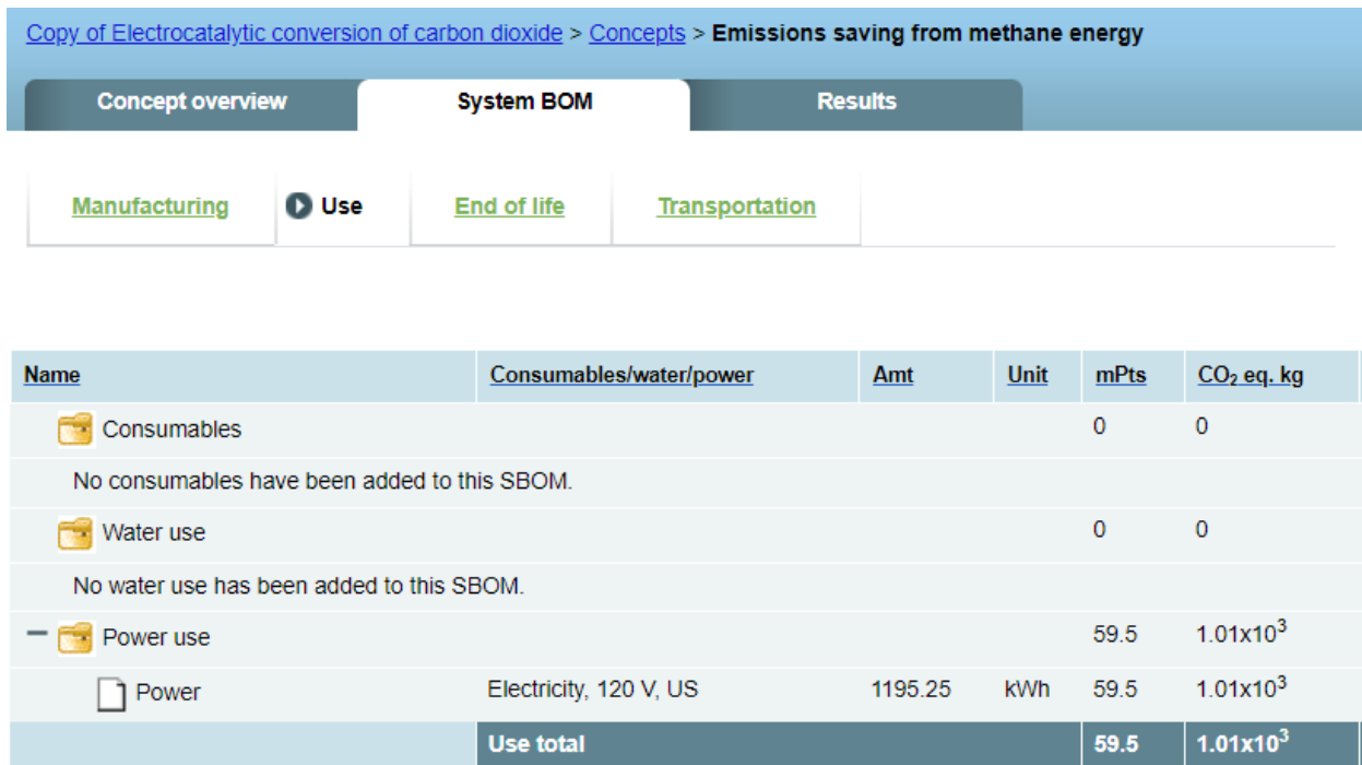
Figure 3.24: Inputs to use phase for estimating emission savings from burning methane generated
