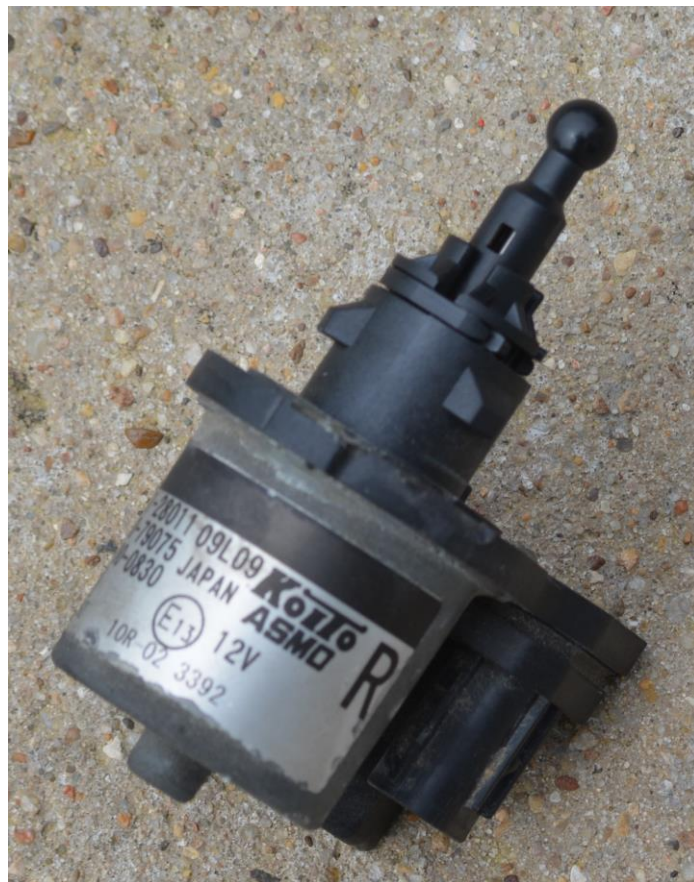
Figure 22 Disassembled Headlight with Linear Actuator Removed
