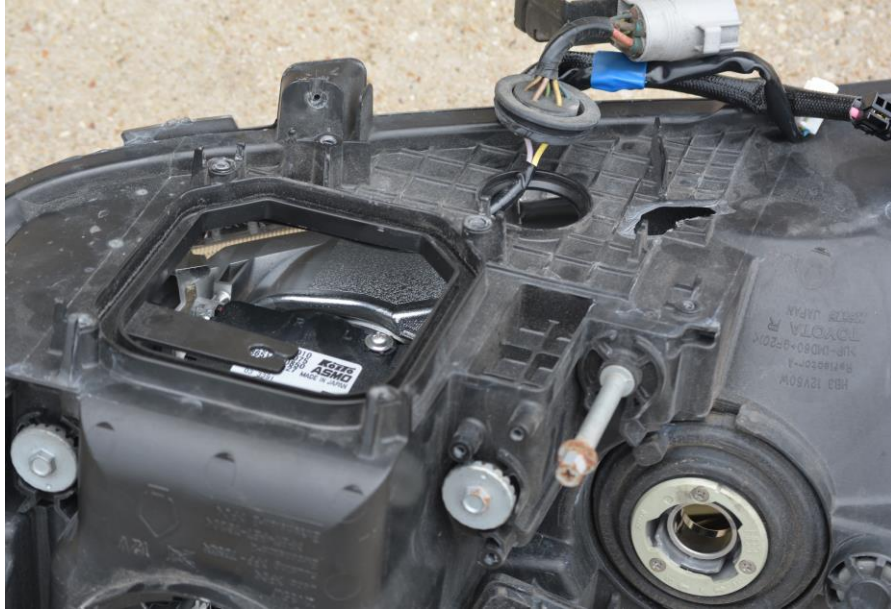
Figure 22 Disassembled Headlight with Linear Actuator Removed
