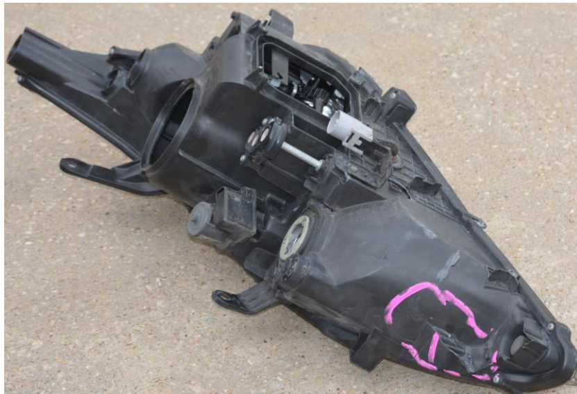
Figure 21 Disassembled Headlight Backside
