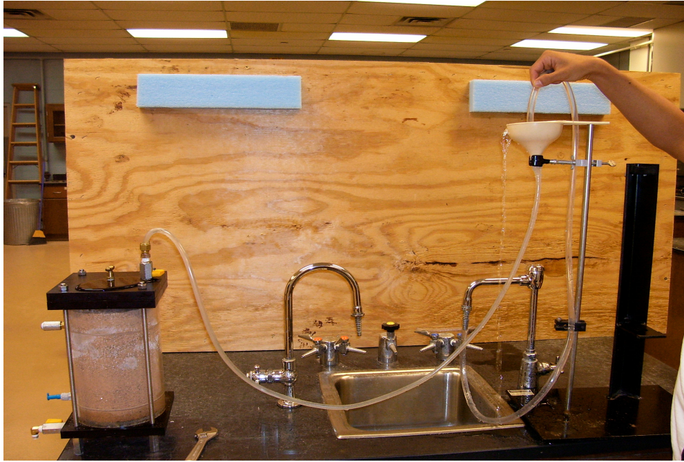
Figure 3.6 Permeability test setup
