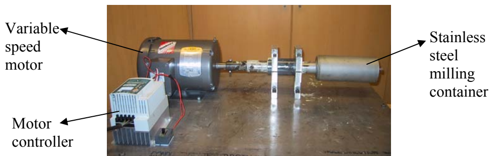
Figure 3.5 The ball milling set up used for milling of NaCl powders
