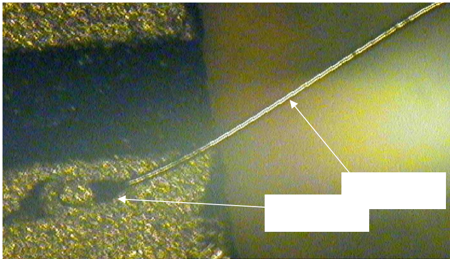
Fig 2.15 Wedge bond on the package lead
