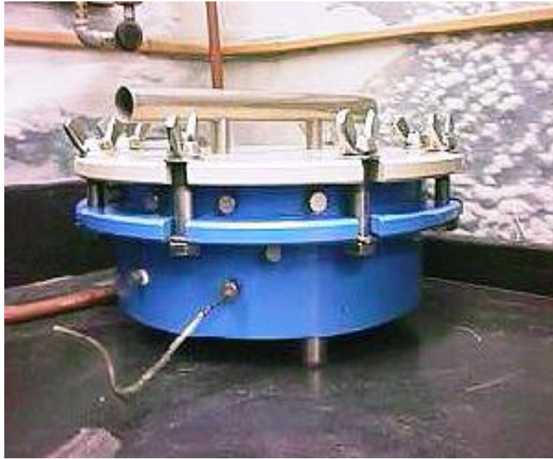
Fig 3.3 15 Bar Extractor Model 1600 (Soil Moisture Corp.).
