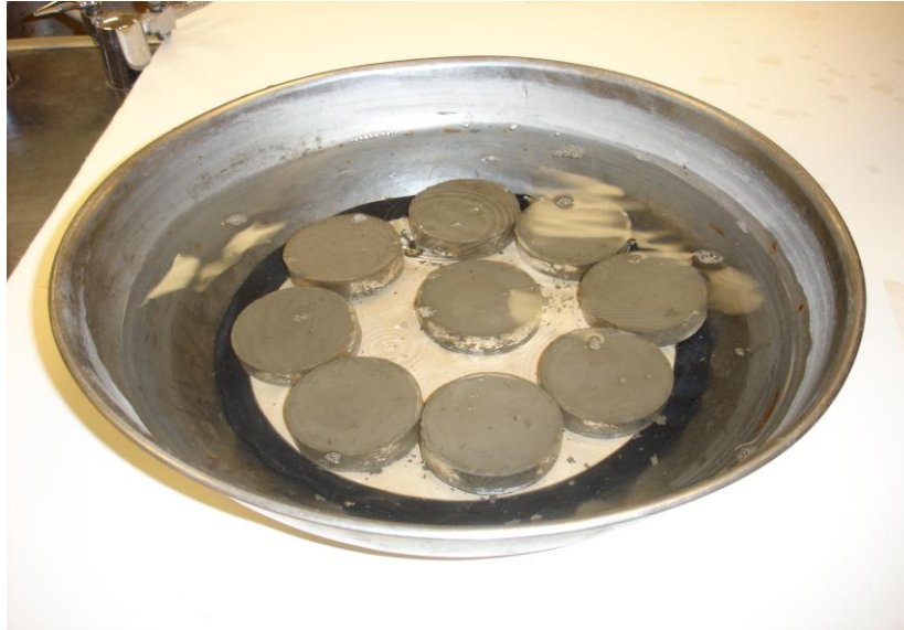
Fig 3.9 Saturation of Soil Specimens.
