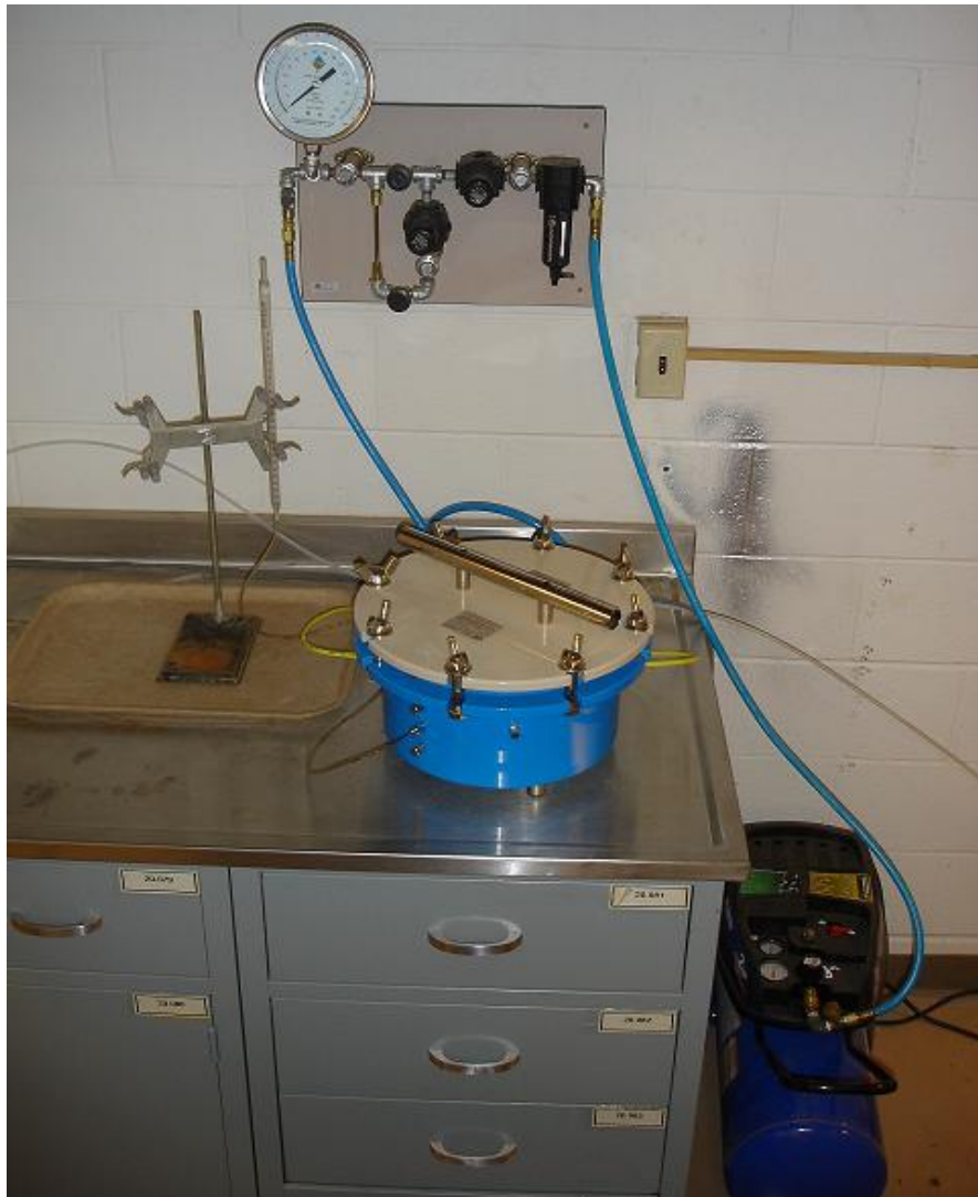
Fig 3.1 Typical Pressure Plate Extractor Setup.
