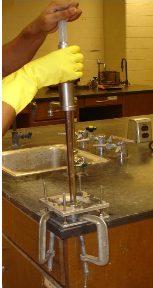
Fig 3.8 Compaction of Soil Specimen.
