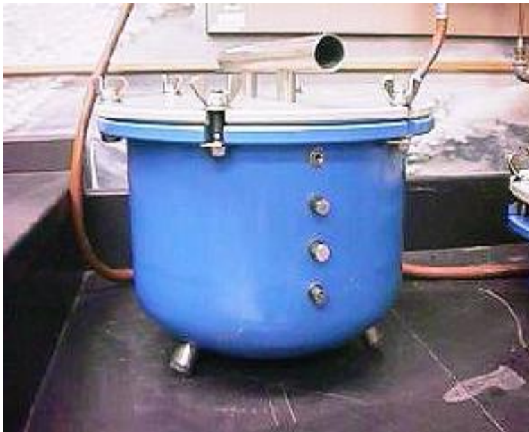
Fig 3.2 5 Bar Extractor Model 1500 (Soil Moisture Corp.).
