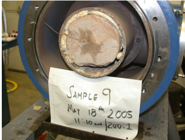
Figure 4.24 Sample 9 in the test section after the test.
