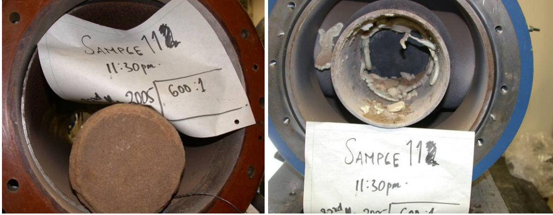
Figure 4.30 Test Section and the cylinder in the nozzle section after the test of Sample 11
