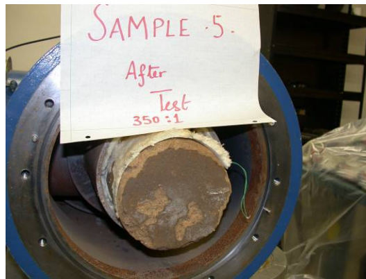
Figure 4.12 Sample 5 in the test section after the test.
