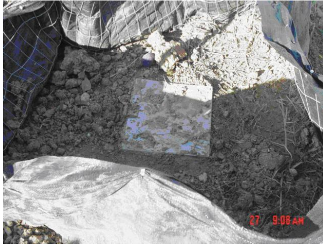
Figure 4.11 Buried Data Box
