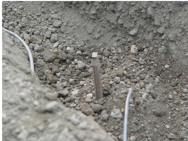
Figure 4.4 Placement of Strain Gauges (Pillappa, 2005)
