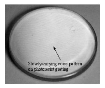
Figure 4.17. Low-frequency noise pattern on a photoresist grating. This noise is due to back-surface reflection from the transparent fused-silica substrate [4, 36].
