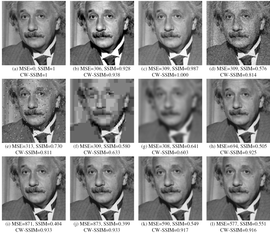
Figure 1.3. Comparison of Image Similarity Measures for Images with Different Types of Distortions. Images are ordered in raster scan. (A) Reference Image (8Bits/Pixel, Assumed To Have Perfect Quality); (B) Contrast Stretch; (C) Mean Luminance Shift; (D) Gaussian Noise Contamination; (E) Impulsive Noise Contamination; (F) JPEG Compression; (G) Blurring; (H) Spatial Scaling (Zooming Out); (I) Spatial Translation (To The Right); (J) Spatial Translation (To The Left); (K) Rotation (Counterclockwise); (L) Rotation (Clockwise).
