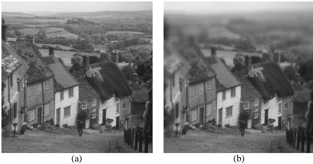
Figure 3.12. Foveated Image (a)Original Image; (b)Foveated Image, where the assumed fixation point is at the man at the lower part of the image.
