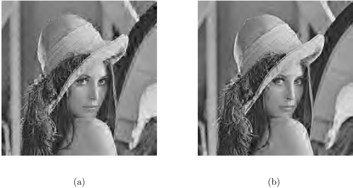
Figure 3.10. Sample image reconstruction for Lena with descriptions loss ratio of 25% (Description 0 is assumed to be lost): (a) image reconstructed by DP-MDC, PSNR = 26.81 dB; (b) image reconstructed by EA-MDC, PSNR = 28.00 dB.
