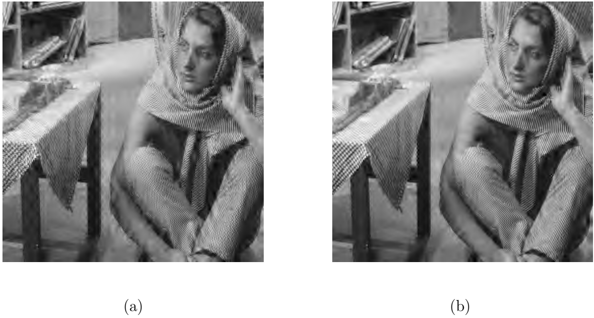
Figure 3.11. Sample image reconstruction for Barbara with descriptions loss ratio of 25% (Description 2 is assumed to be lost): (a) image reconstructed by DP-MDC, PSNR = 24.30 dB; (b) image reconstructed by EA-MDC, PSNR = 25.97 dB.
