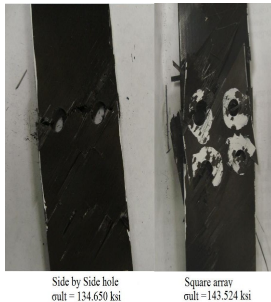
Figure 4.9 Failure comparisons of laminates with SSH & SA pattern
